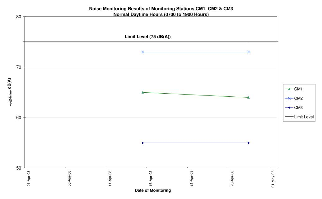
Note: (1) CM2 is a non-façade measurement location. A positive correction of 3dB(A) has been applied to the measured noise level according to EPD's guideline.
