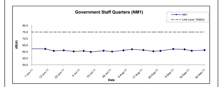
Title Contract No. DC/2009/09 Construction of Tai Po Sewage Treatment Works - Stage V Phase II B **Graphical Presentation of Construction Noise Monitoring**
