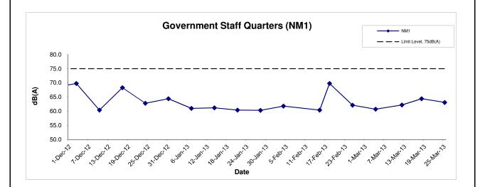
Scale Project Contract No. DC/2009/09 No. Construction of Tai Po Sewage Treatment Works - Stage V Phase II B N.T.S MA10069 Appendix Date Graphical Presentation of Construction Noise Monitoring Mar 13 Results
