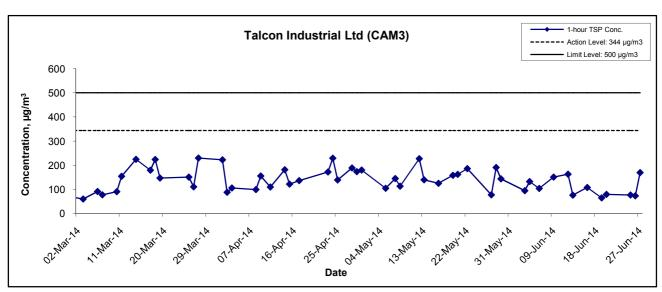
Title Contract No. DC/2009/09 No. Construction of Tai Po Sewage Treatment Works - Stage V Phase II B N.T.S Date Graphical Presentation of 1-hour TSP Impact Monitoring Jun 14 Results
