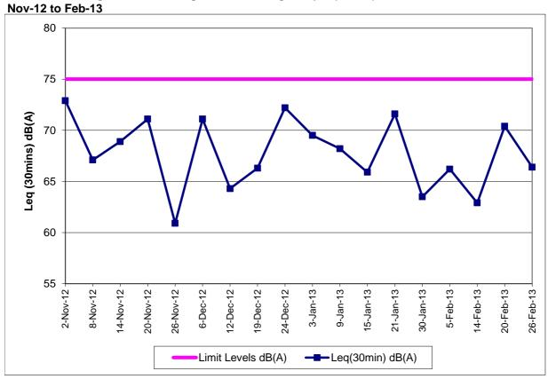
Contract No. DC/2007/12 - Design and Construction of Tsuen Wan Drainage Tunnel Noise Monitoring Results at Squatters (NSR 6)
