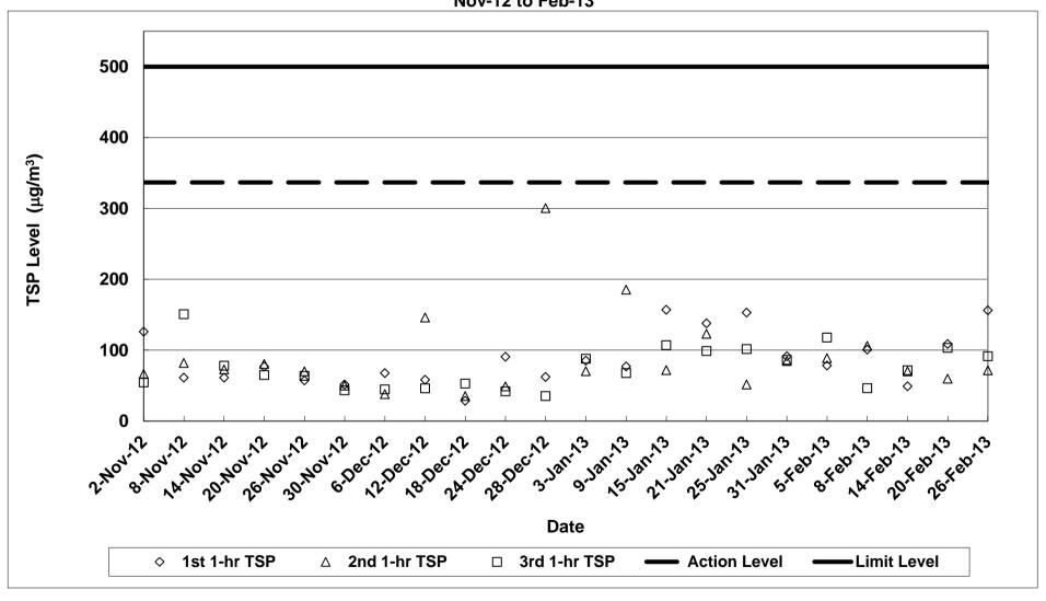
Contract No. DC/2007/12 - Design and Construction of Tsuen Wan Drainage Tunnel Air Quality Monitoring (1-hr TSP) Results at Greenview Terrace - Outfall (ASR9)
