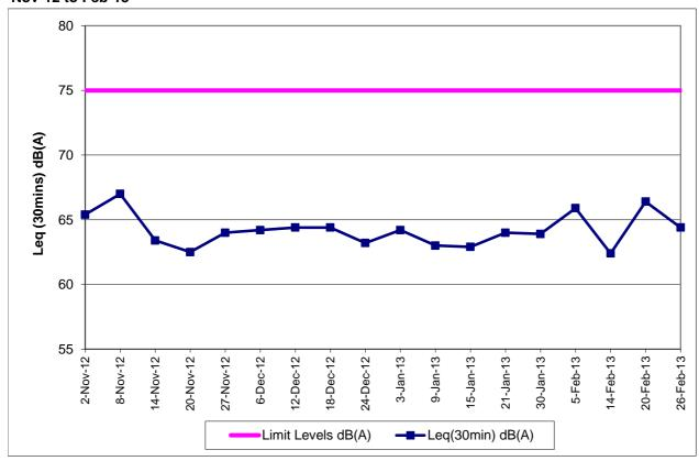
Contract No. DC/2007/12 - Design and Construction of Tsuen Wan Drainage Tunnel Noise Monitoring Results at Greenview Terrace (NSR 9)
