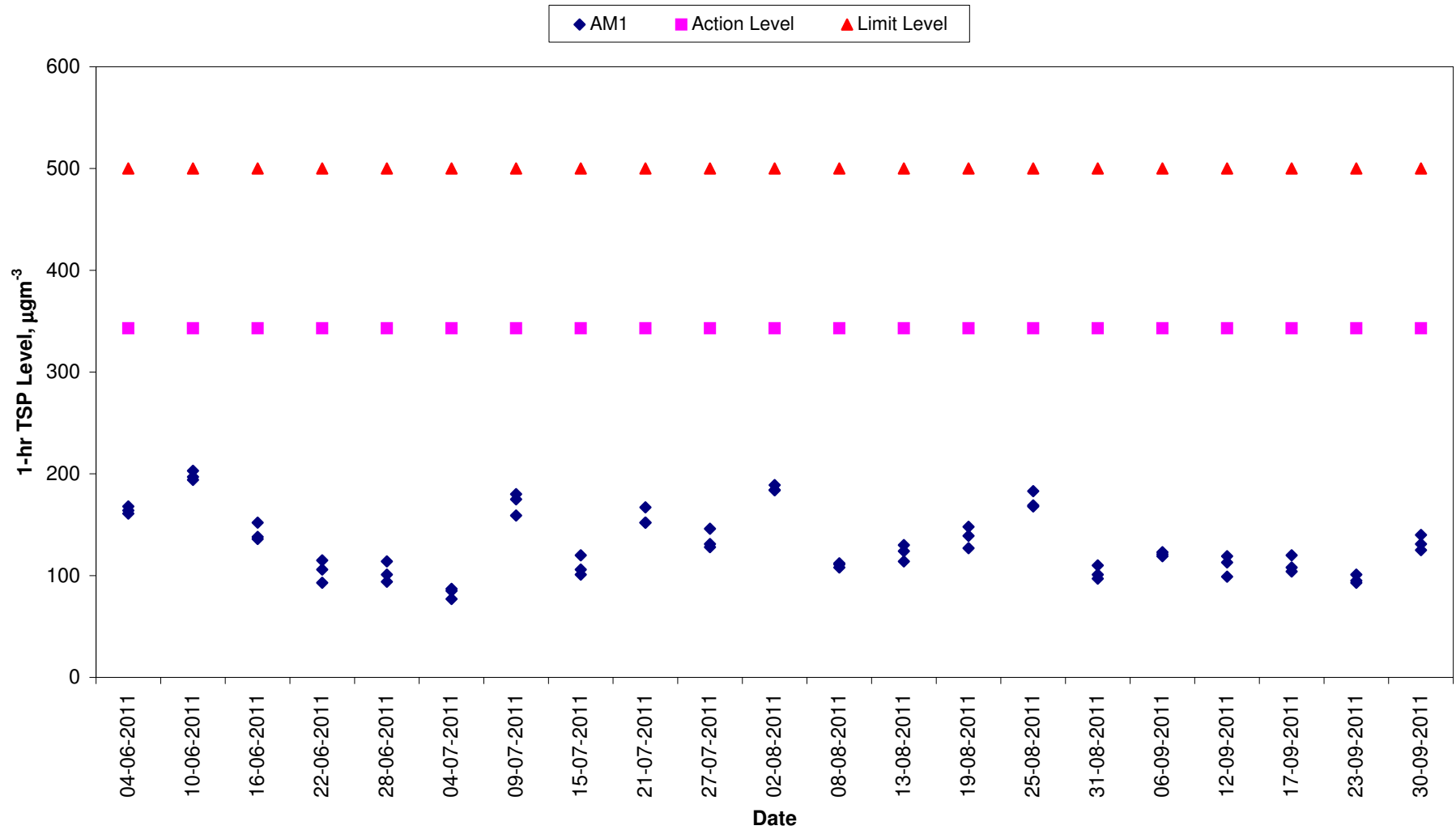
1-hr TSP Levels for the Past 4 Months AM1 (Tuen Mun EMSD Vehicle Servicing Station)
