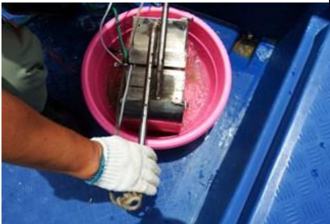
Photo3. Grab sampler and sediment-benthic sample
