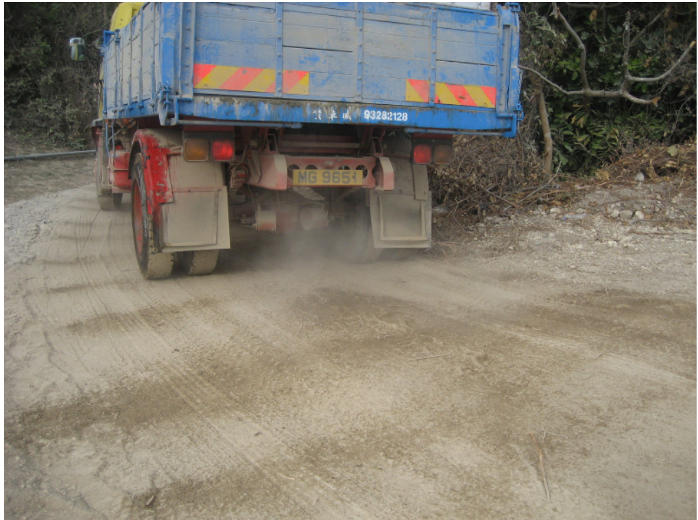
Photo 1 – Dust was generated at haul road when trucks leaving the site at the exit of Site 1.
