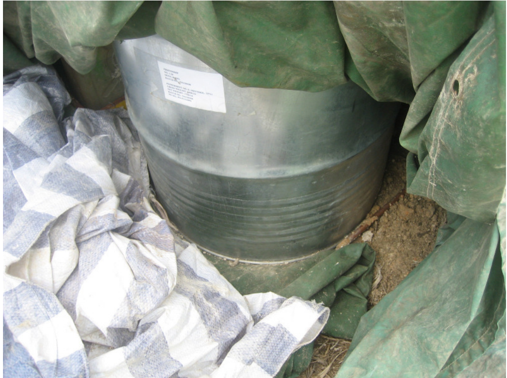
Photo 1 – An oil drum was observed storing without drip tray at Site 1.
