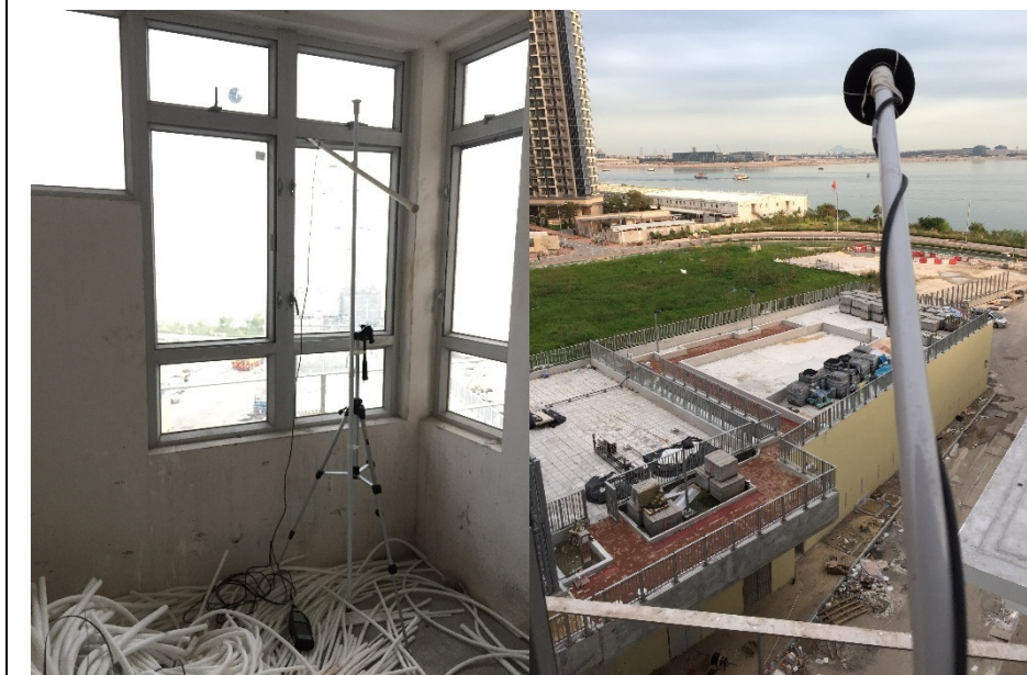
Photo 2 – Noise Measurement Setup
