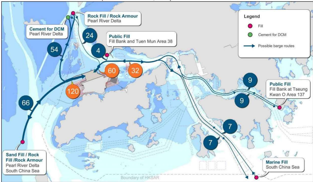
Figure 5-2 Indicative Marine Travel Route with Forecast Construction Traffic Movements during Peak Period per Day after Commencement of Reclamation before the Operation of Interim 2RS (modified from BMT, 2014)
