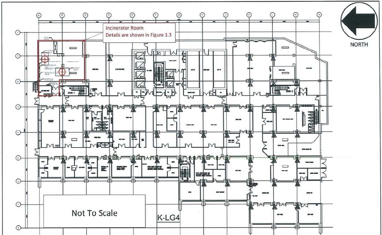
FIGURE 1.2 LG4/F LAYOUT PLAN OF BLOCK K SHOWING THE LOCATION OF THE INCINERATOR ROOM
