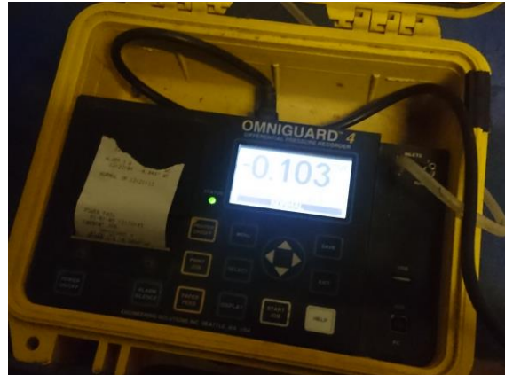
Figure 3.15 Pressure monitor was kept within the normal range during smoke test
