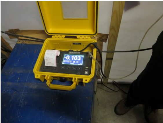
Figure 3.8 Pressure monitor with audible alarm and records printing out
