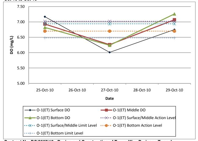
Contract No. DC/2007/12 - Design and Construction of Tsuen Wan Drainage Tunnel Water Quality Results at Control of Outfall 1 During Ebb Tide (O-1-C(ET)) Oct-10 to Oct-10
