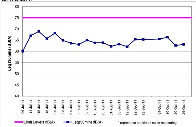
Contract No. DC/2007/12 - Design and Construction of Tsuen Wan Drainage Tunnel Noise Monitoring Results at Long Beach Gardens (NSR 8) Jul-11 to Oct-11
