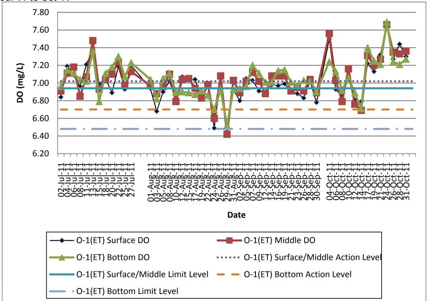
Contract No. DC/2007/12 - Design and Construction of Tsuen Wan Drainage Tunnel Water Quality Results at Control of Outfall 1 During Ebb Tide (O-1-C(ET)) Jul-11 to Oct-11
