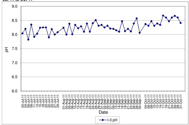
Contract No. DC/2007/12 - Design and Construction of Tsuen Wan Drainage Tunnel Water Quality Results at Squatters (I-3-C)
