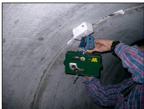
Figure 15. Automatic camera was installed inside the underpass crossing underneath the Route 3 to monitor the wildlife uses of the tunnel.
