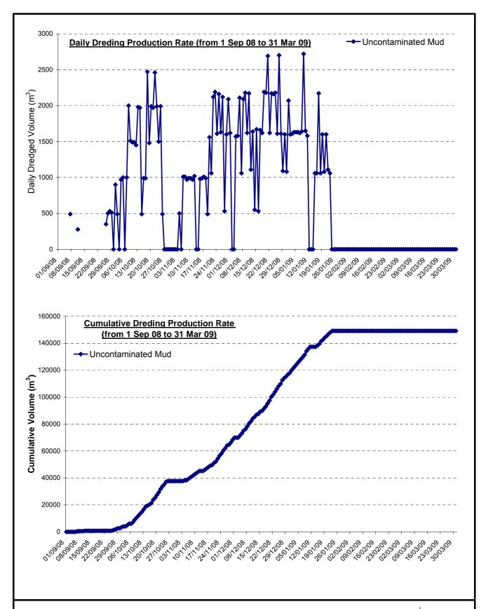
Figure 2.1 Daily and cumulative volumes (m³) of excavated materials from 1 September to 31 March 2009. Excavated materials contained uncontaminated mud only.
