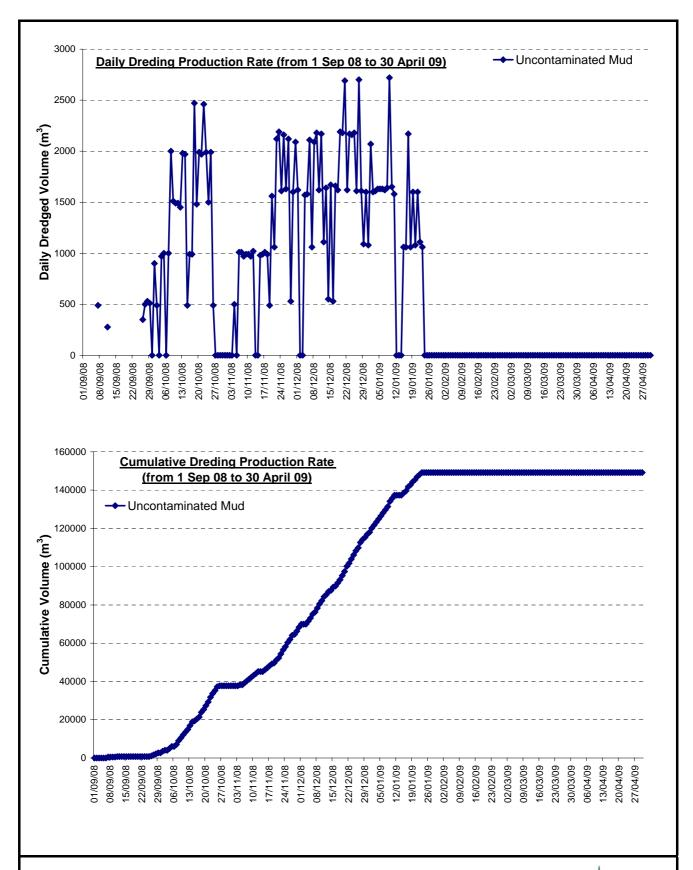
Figure 2.1 Daily and cumulative volumes (m³) of excavated materials from 1 September to 30 April 2009. Excavated materials contained uncontaminated mud only.
