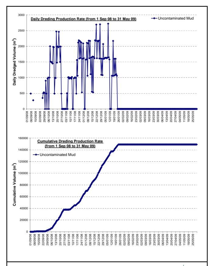
Figure 2.1 Daily and cumulative volumes (m³) of excavated materials from 1 September to 31 May 2009. Excavated materials contained uncontaminated mud only.
