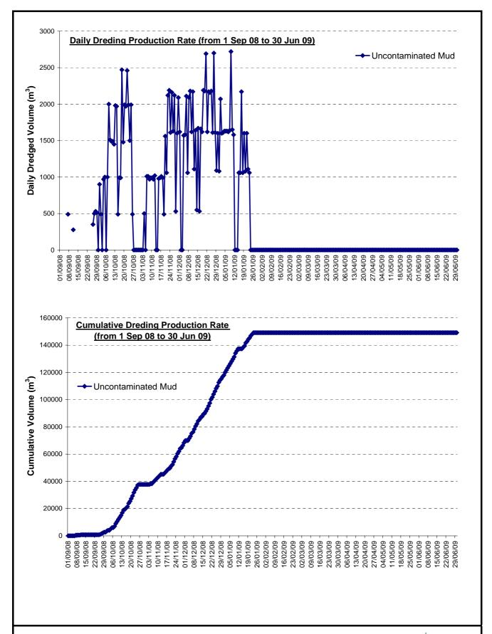
Figure 2.1 Daily and cumulative volumes (m³) of excavated materials from 1 September to 30 June 2009. Excavated materials contained uncontaminated mud only.
