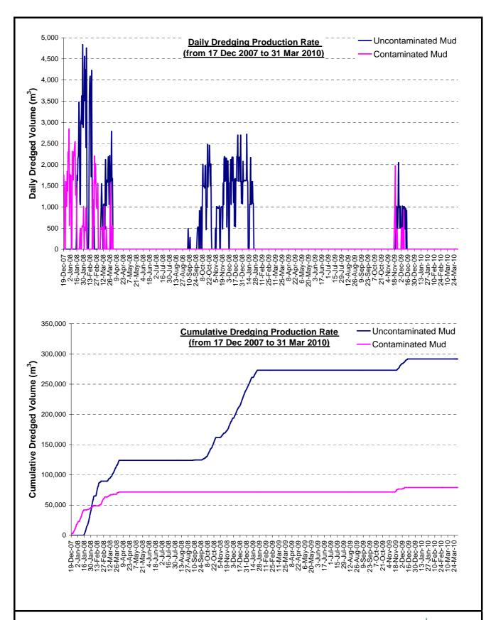
Figure 2.1 Daily and cumulative volumes (m³) of excavated materials (both contaminated and uncontaminated mud) from 19 December 2007 to 31 March 2010
