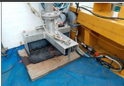
Plate 7: The transducer of the R2Sonic Sonic 2024 multibeam echo sounding system
