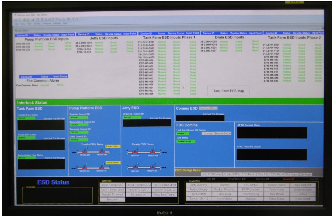
(31) The ESD regular testing as shown in SCADA System
