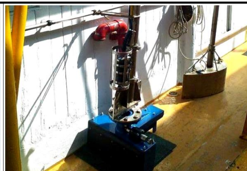
Plate 7: The transducer of the multibeam echo sounding system
