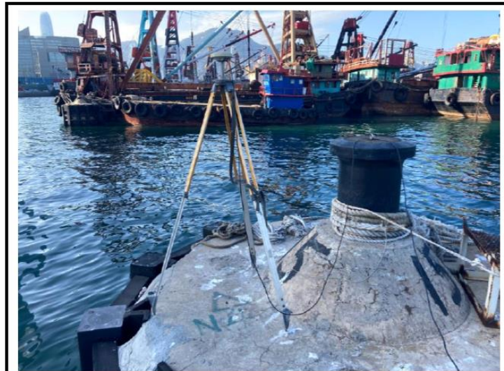
Plate 4: DGPS check at Tuen Mun Typhoon Shelter
