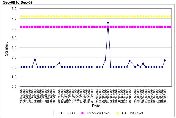
Contract No. DC/2007/12 - Design and Construction of Tsuen Wan Drainage Tunnel Water Quality Results at Squatters (I-3-C) Sep-09 to Dec-09
