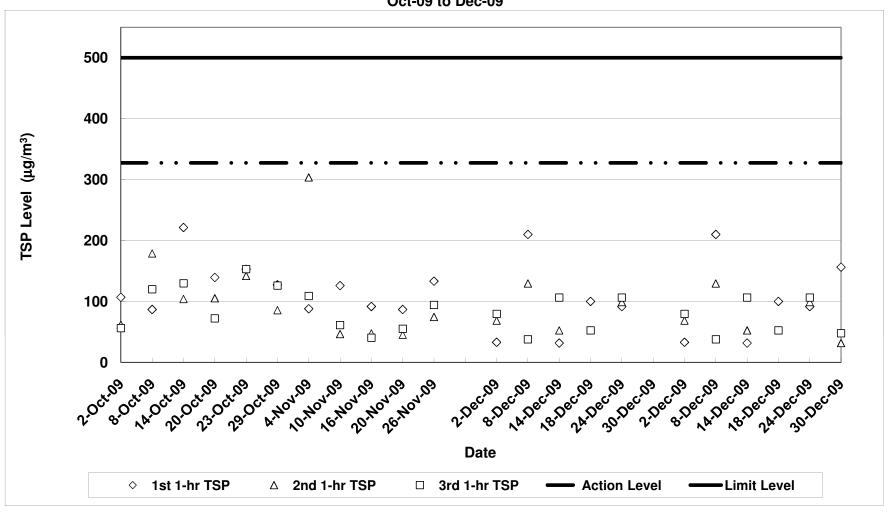
Contract No. DC/2007/12 - Design and Construction of Tsuen Wan Drainage Tunnel Air Quality Monitoring (1-hr TSP) Results at Long Beach Gardens - Outfall (ASR8)
