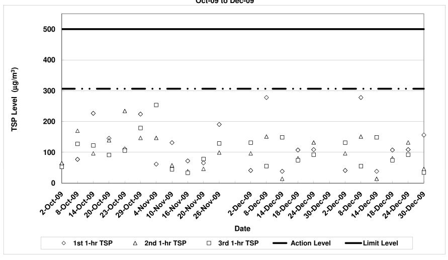
Contract No. DC/2007/12 - Design and Construction of Tsuen Wan Drainage Tunnel Air Quality Monitoring (1-hr TSP) Results at Hong Hoi Chee Hong Temple - Intake (ASR3) Oct-09 to Dec-09
