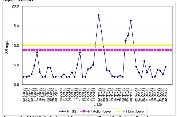
Contract No. DC/2007/12 - Design and Construction of Tsuen Wan Drainage Tunnel Water Quality Results at Sik Sik Yuen Ho Fung College (I-1-C) Sep-09 to Dec-09
