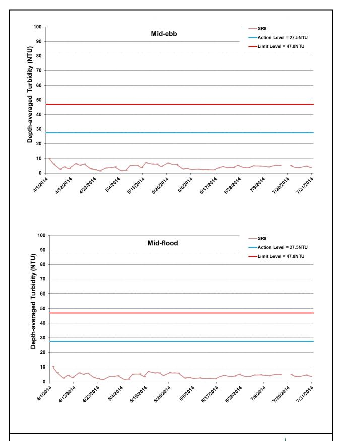
Figure I33 Impact Monitoring – Mean Depth-averaged Level of Turbidity (NTU) between 1 April 2014 and 31 July 2014 at SR8. The weather conditions during the monitoring period varied mostly from sunny to cloudy. Major marine construction activities included: Dredging (4/1/2014 – 7/31/2014); Construction of Temporary Seawalls (4/1/2013 – 7/31/2014); Sheet Piling (4/1/2014 – 7/31/2014); Filling (4/1/2014 – 7/31/2014). No monitoring was conducted on 18 July 2014 due to adverse weather condition.
