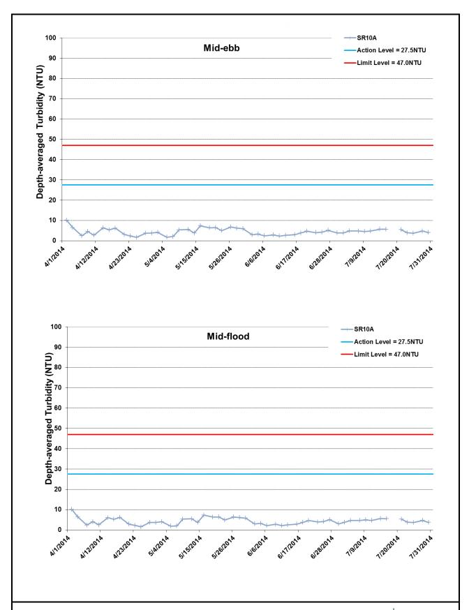
Figure I32 Impact Monitoring – Mean Depth-averaged Level of Turbidity (NTU) between 1 April 2014 and 31 July 2014 at SR10A. The weather conditions during the monitoring period varied mostly from sunny to cloudy. Major marine construction activities included: Dredging (4/1/2014 – 7/31/2014); Construction of Temporary Seawalls (4/1/2013 – 7/31/2014); Sheet Piling (4/1/2014 – 7/31/2014); Filling (4/1/2014 – 7/31/2014). No monitoring was conducted on 18 July 2014 due to adverse weather condition.
