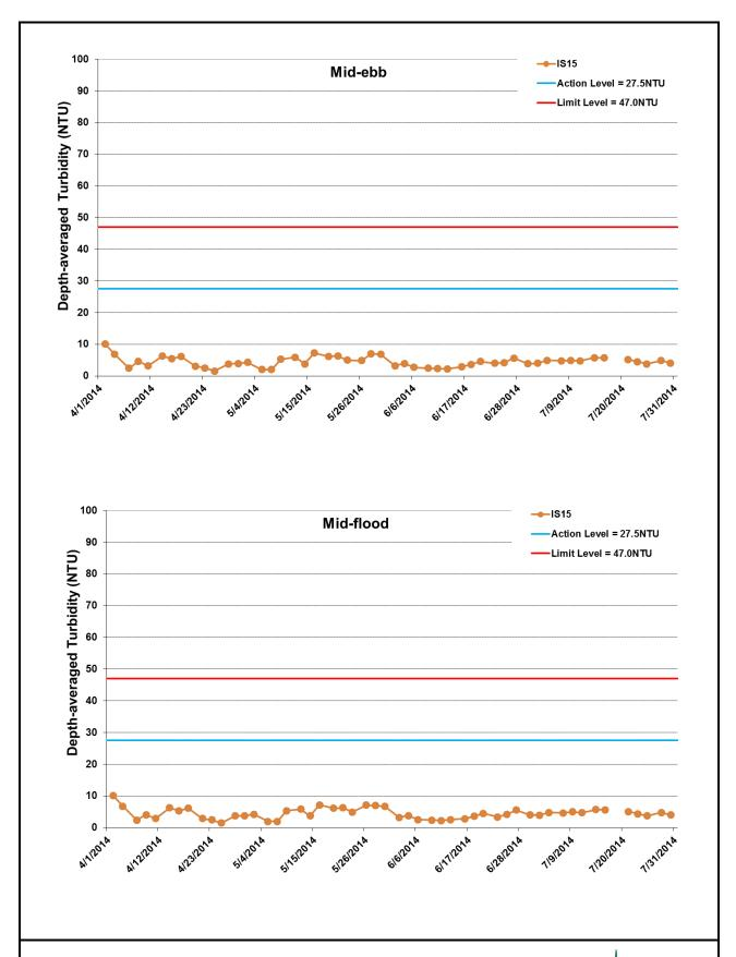
Figure I31 Impact Monitoring – Mean Depth-averaged Level of Turbidity (NTU) between 1 April 2014 and 31 July 2014 at IS15. The weather conditions during the monitoring period varied mostly from sunny to cloudy. Major marine construction activities included: Dredging (4/1/2014 – 7/31/2014); Construction of Temporary Seawalls (4/1/2013 – 7/31/2014); Sheet Piling (4/1/2014 – 7/31/2014); Filling (4/1/2014 – 7/31/2014). No monitoring was conducted on 18 July 2014 due to adverse weather condition.
