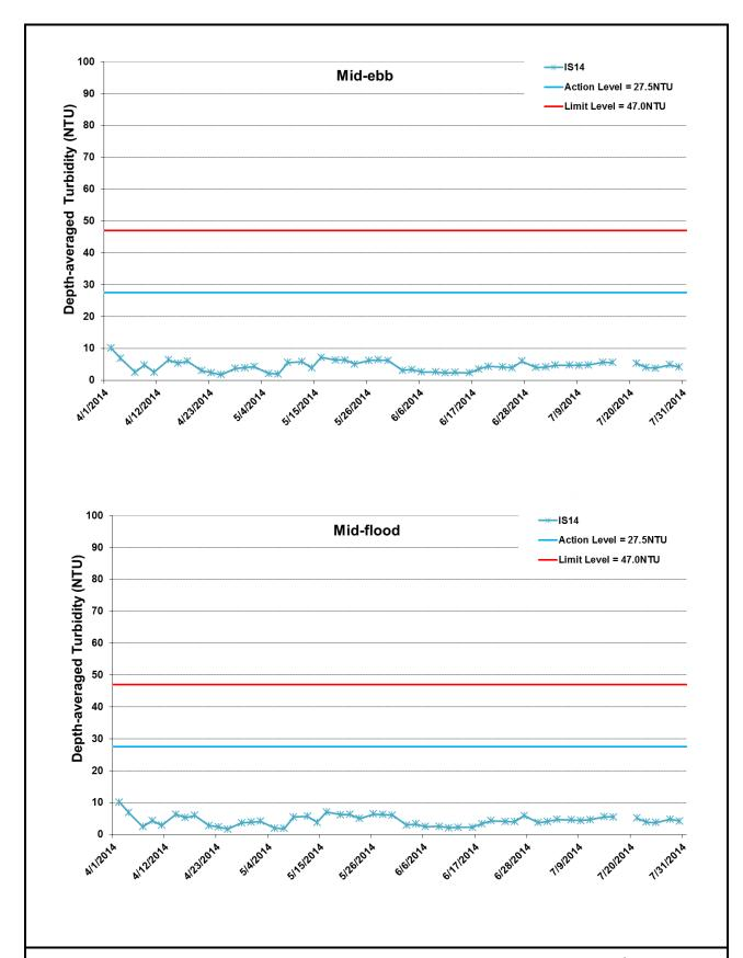
Figure I30 Impact Monitoring – Mean Depth-averaged Level of Turbidity (NTU) between 1 April 2014 and 31 July 2014 at IS14. The weather conditions during the monitoring period varied mostly from sunny to cloudy. Major marine construction activities included: Dredging (4/1/2014 – 7/31/2014); Construction of Temporary Seawalls (4/1/2013 – 7/31/2014); Sheet Piling (4/1/2014 – 7/31/2014); Filling (4/1/2014 – 7/31/2014). No monitoring was conducted on 18 July 2014 due to adverse weather condition.
