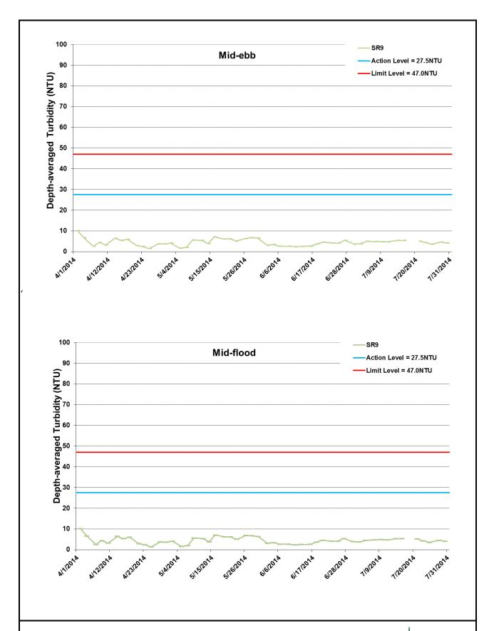
Figure I34 Impact Monitoring – Mean Depth-averaged Level of Turbidity (NTU) between 1 April 2014 and 31 July 2014 at SR9. The weather conditions during the monitoring period varied mostly from sunny to cloudy. Major marine construction activities included: Dredging (4/1/2014 – 7/31/2014); Construction of Temporary Seawalls (4/1/2013 – 7/31/2014); Sheet Piling (4/1/2014 – 7/31/2014); Filling (4/1/2014 – 7/31/2014). No monitoring was conducted on 18 July 2014 due to adverse weather condition.
