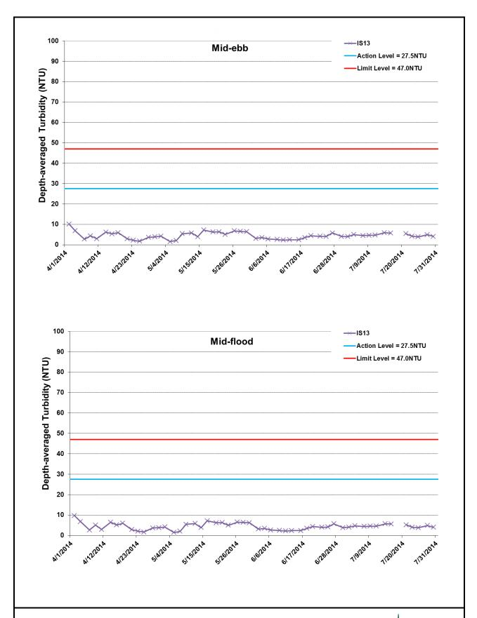
Figure I29 Impact Monitoring – Mean Depth-averaged Level of Turbidity (NTU) between 1 April 2014 and 31 July 2014 at IS13. The weather conditions during the monitoring period varied mostly from sunny to cloudy. Major marine construction activities included: Dredging (4/1/2014 – 7/31/2014); Construction of Temporary Seawalls (4/1/2013 – 7/31/2014); Sheet Piling (4/1/2014 – 7/31/2014); Filling (4/1/2014 – 7/31/2014). No monitoring was conducted on 18 July 2014 due to adverse weather condition.
