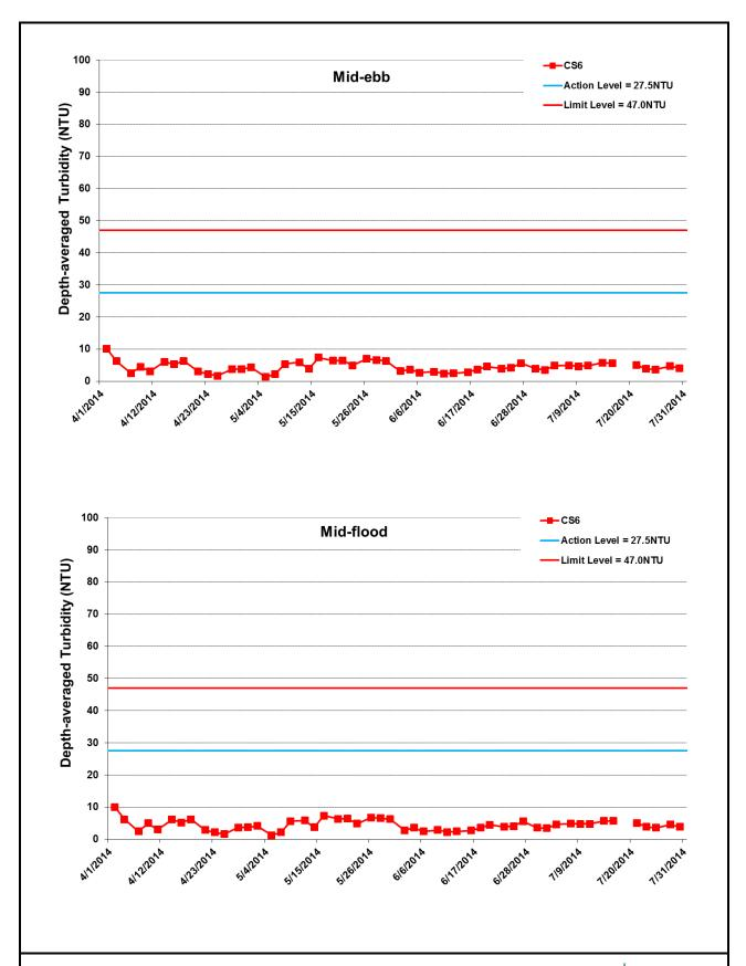
Figure I27 Impact Monitoring – Mean Depth-averaged Level of Turbidity (NTU) between 1 April 2014 and 31 July 2014 at CS6. The weather conditions during the monitoring period varied mostly from sunny to cloudy. Major marine construction activities included: Dredging (4/1/2014 – 7/31/2014); Construction of Temporary Seawalls (4/1/2013 – 7/31/2014); Sheet Piling (4/1/2014 – 7/31/2014); Filling (4/1/2014 – 7/31/2014). No monitoring was conducted on 18 July 2014 due to adverse weather condition.
