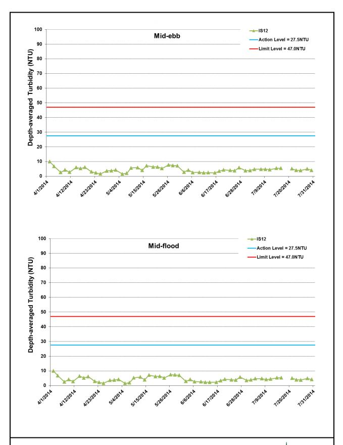
Figure I28 Impact Monitoring – Mean Depth-averaged Level of Turbidity (NTU) between 1 April 2014 and 31 July 2014 at IS12. The weather conditions during the monitoring period varied mostly from sunny to cloudy. Major marine construction activities included: Dredging (4/1/2014 – 7/31/2014); Construction of Temporary Seawalls (4/1/2013 – 7/31/2014); Sheet Piling (4/1/2014 – 7/31/2014); Filling (4/1/2014 – 7/31/2014). No monitoring was conducted on 18 July 2014 due to adverse weather condition.
