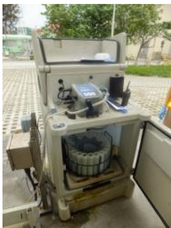
Photo 4-1 Hach Sigma AWRS Sampler
