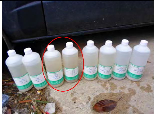
Photo 2 The water samples collected at WM2B was visually turbid on 16 January 2016.
