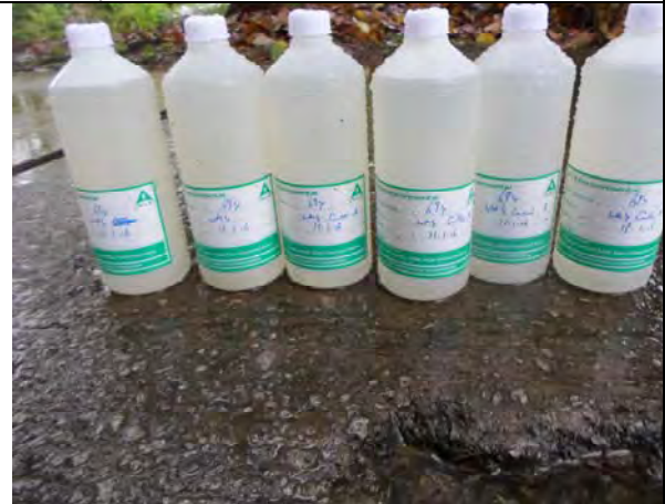
Photo 4 The water samples collected at WM4, WM4-CA and WM4-CB on 15 January 2016 were turbid.
