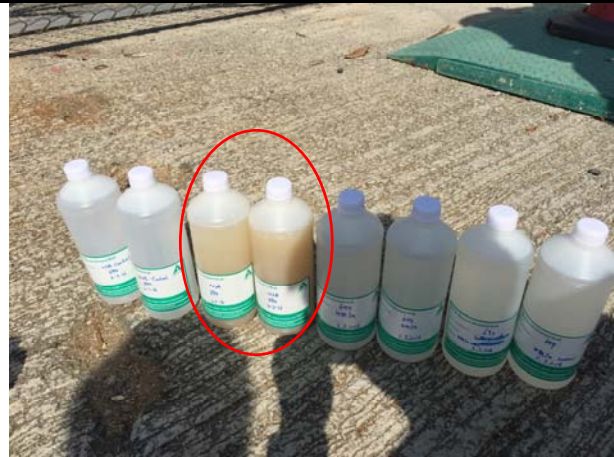
Photo 2 The water samples collected at WM2B on 2 March 2016 was turbid.
