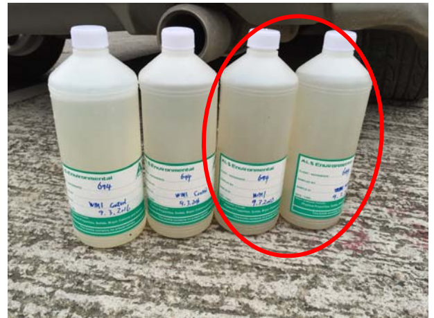
Photo 6 The water samples collected at both WM1-C and WM1 on 9 March 2016 were slightly turbid.
