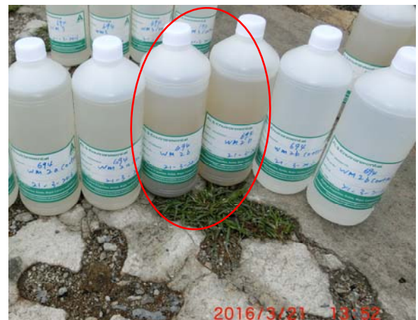
Photo 2 The water samples collected at WM2B on 21 March 2016 was turbid.
