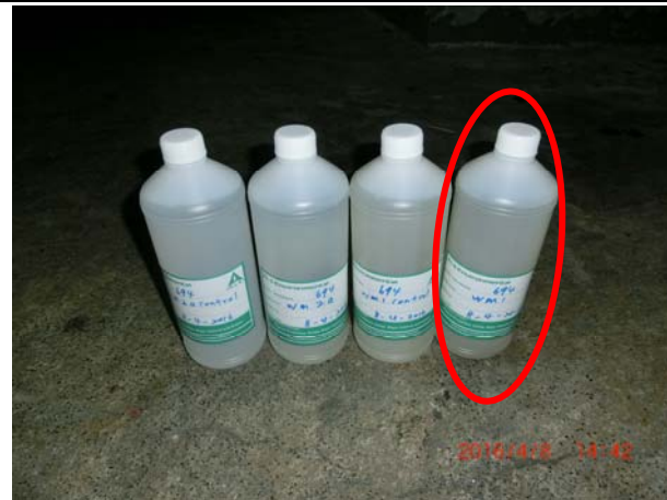
Photo 15 The water samples collected at WM1 on 8 April 2016 were slightly turbid.
