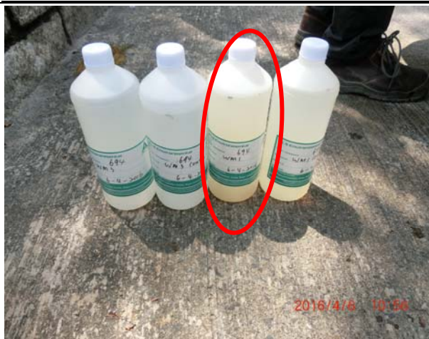
Photo 7 The water samples collected at WM1 on 6 April 2016 were slightly turbid.
