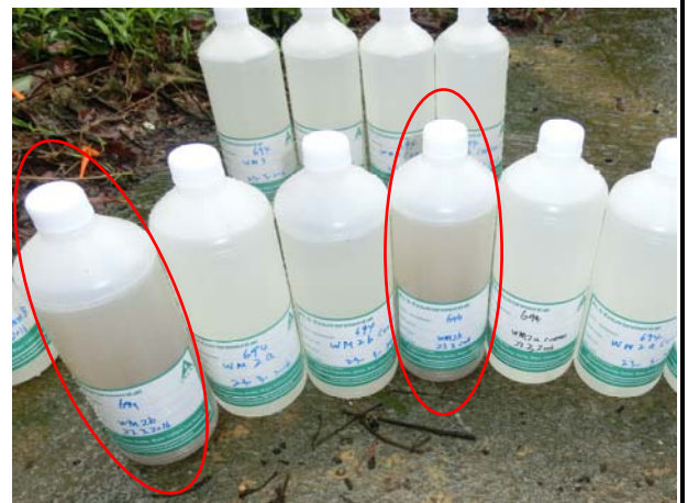
Photo 2 The water samples collected at WM2B on 23 March 2016 was turbid.
