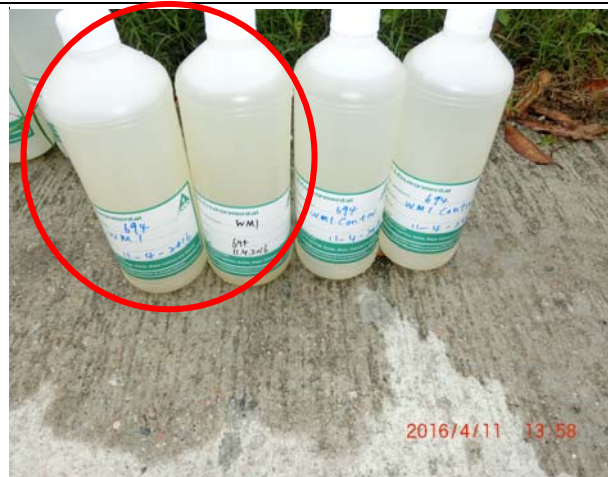
Photo 3 The water samples collected at WM1 on 11 April 2016 were slightly turbid.
