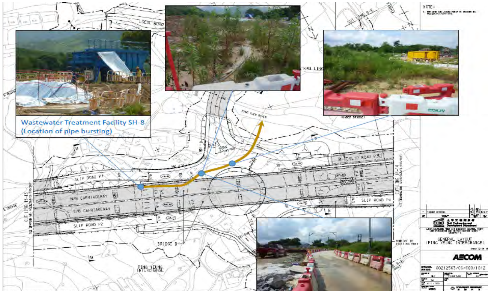
Figure 1 The layout for the path of runoff into the Ping Yuen River due to the pipe burst
