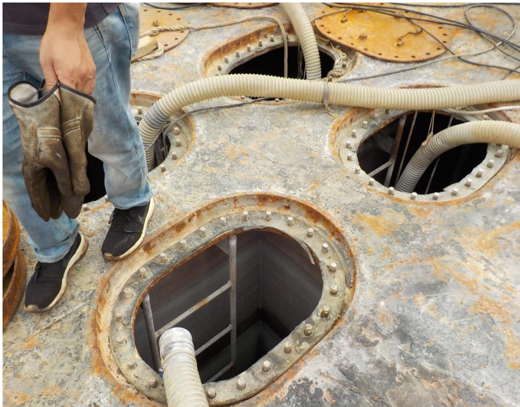
Ballast water is pumped in and out of the ballast tank.
