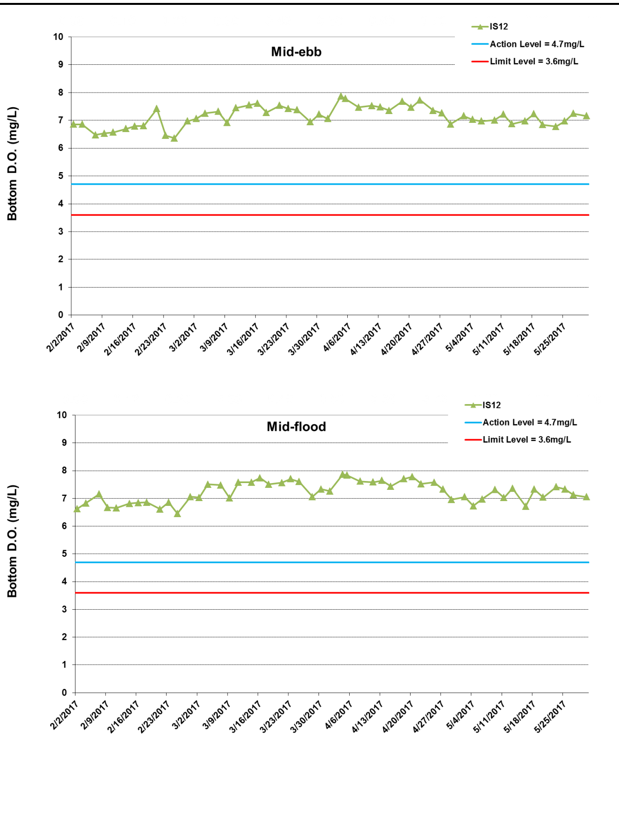
Figure G19 Impact Monitoring - Mean Level of Dissolved Oxygen (mg/L) in bottom water between 1 February 2017 and 31 May 2017 at IS12. The weather conditions during the monitoring period varied mostly from sunny to cloudy. Major marine works included: Filling works at Portion N-A (1/3/2017 - 20/5/2017).
