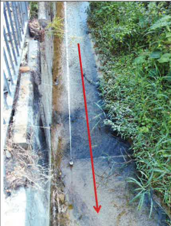
Photo 2 View of upstream of Location WM2B The water depth is approximately 0.01-0.02m.
