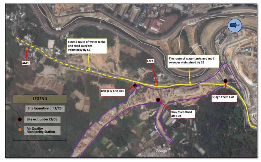
Figure 1 Layout of Air Quality Monitoring Locations AM2 and AM3
