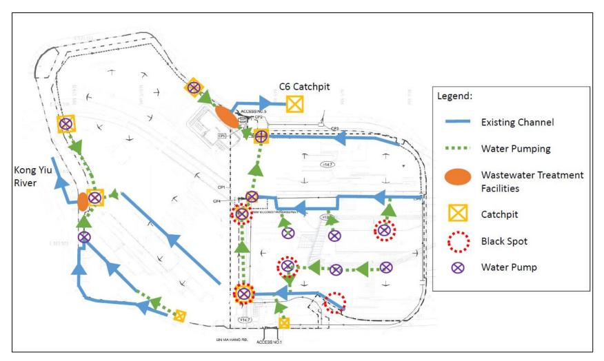
Figure 2 layout of Temporary drainage system for SS C505
