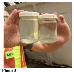
On-site water test for pH value and visual test for suspended solids were carried out for water retained in the recycling tank (eventually overflow off site) and no abnormal results was found in these reference test.
