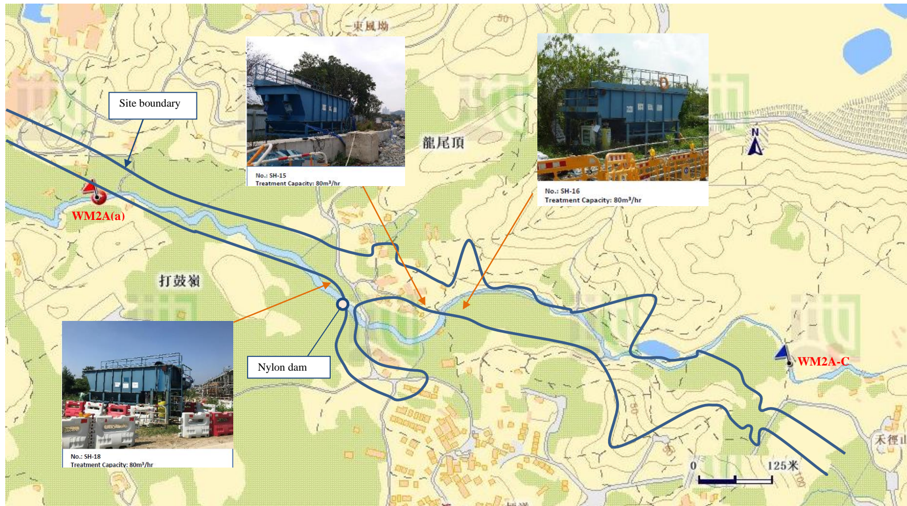
Figure 1 Location Map for Water Quality Monitoring Locations WM2A(a), WM2A-Control and work area under Contract 6
