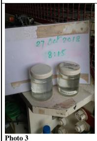
DHK conducted self-checking on the effluent quality of wastewater treatment facility at North Portal Site on 27 Oct 2018. DHK reported that the visual test result revealed that the quality of discharge was acceptable under supervision by RE.
