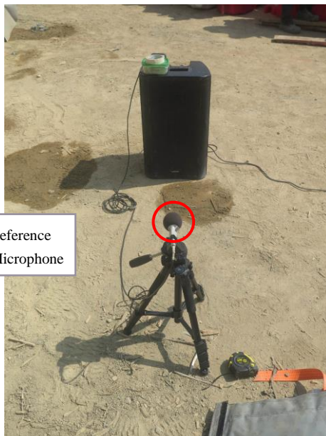
Photo A3. Loudspeaker and Reference Microphone for without Noise Barrier Scenario
