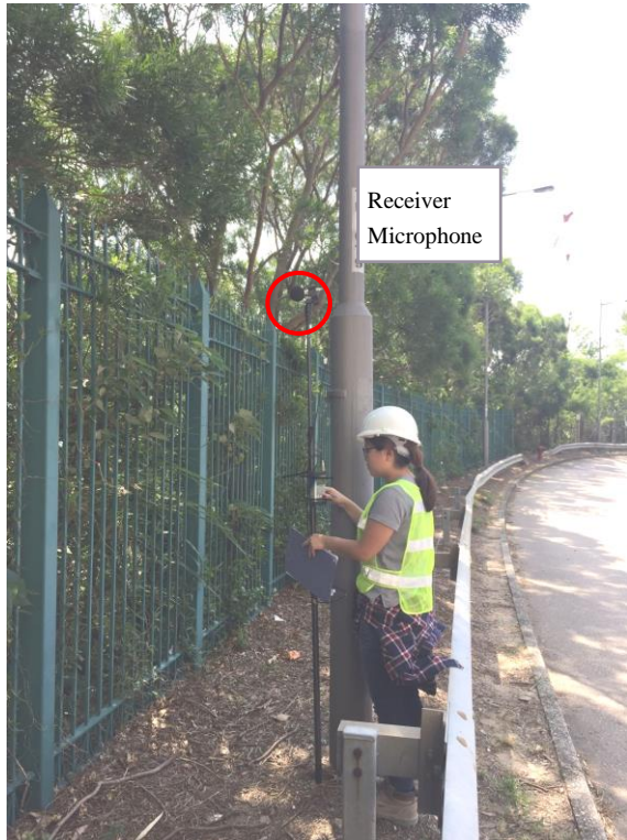
Photo A1. Receiver Microphone
