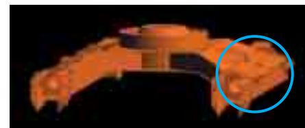
Undercarriage Designed for Easy Mud Removal
