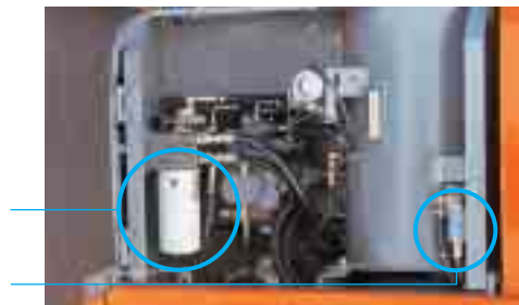
Engine Oil Filter and Water Separator Positioned for Easy Checking from Ground
