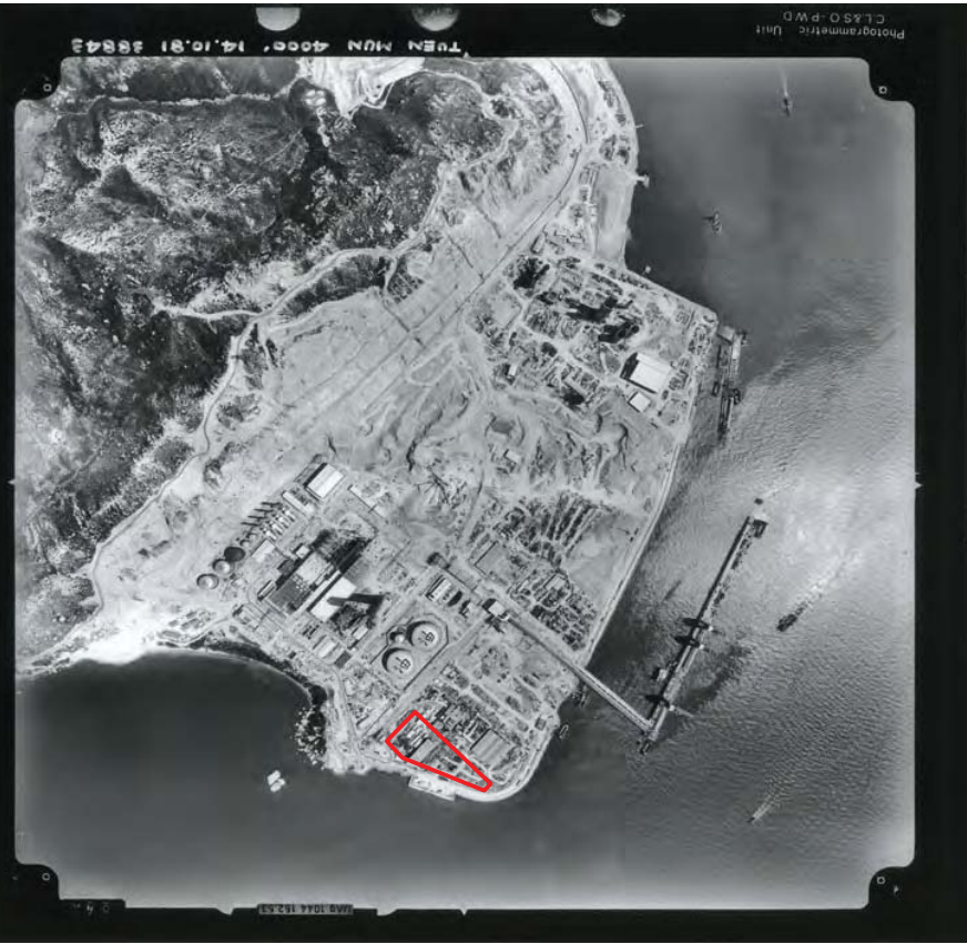
Year 1981 (ref: 38843): Reclamation is completed and the CPPS was under construction. Constructions (Temporary low-rise housing structures / container offices / workshops) were found within the southern part of the works area.
