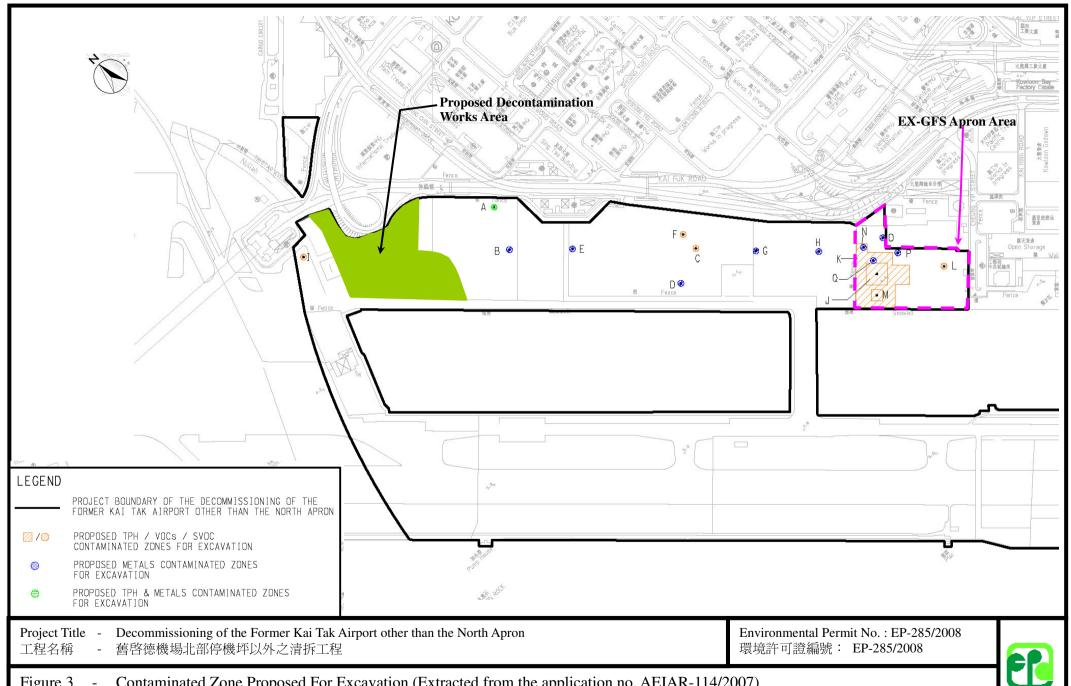
Contaminated Zone Proposed For Excavation (Extracted from the application no. AEIAR-114/2007) Figure 3
