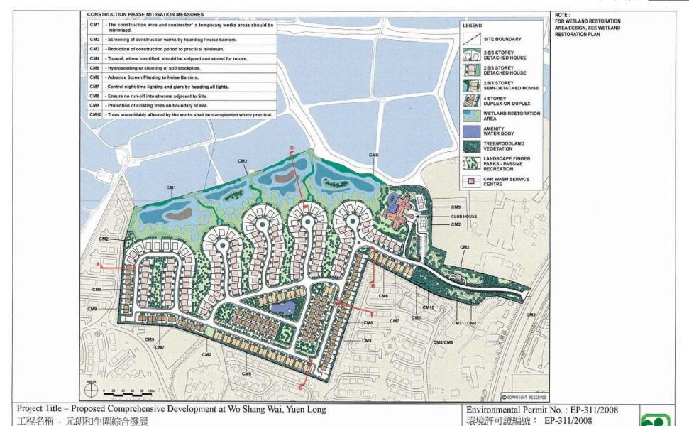
Figure 4 – Landscape and Visual Mitigation Measures during Construction Phase 圖 4 -施工期間的景觀及視覺緩解措施
