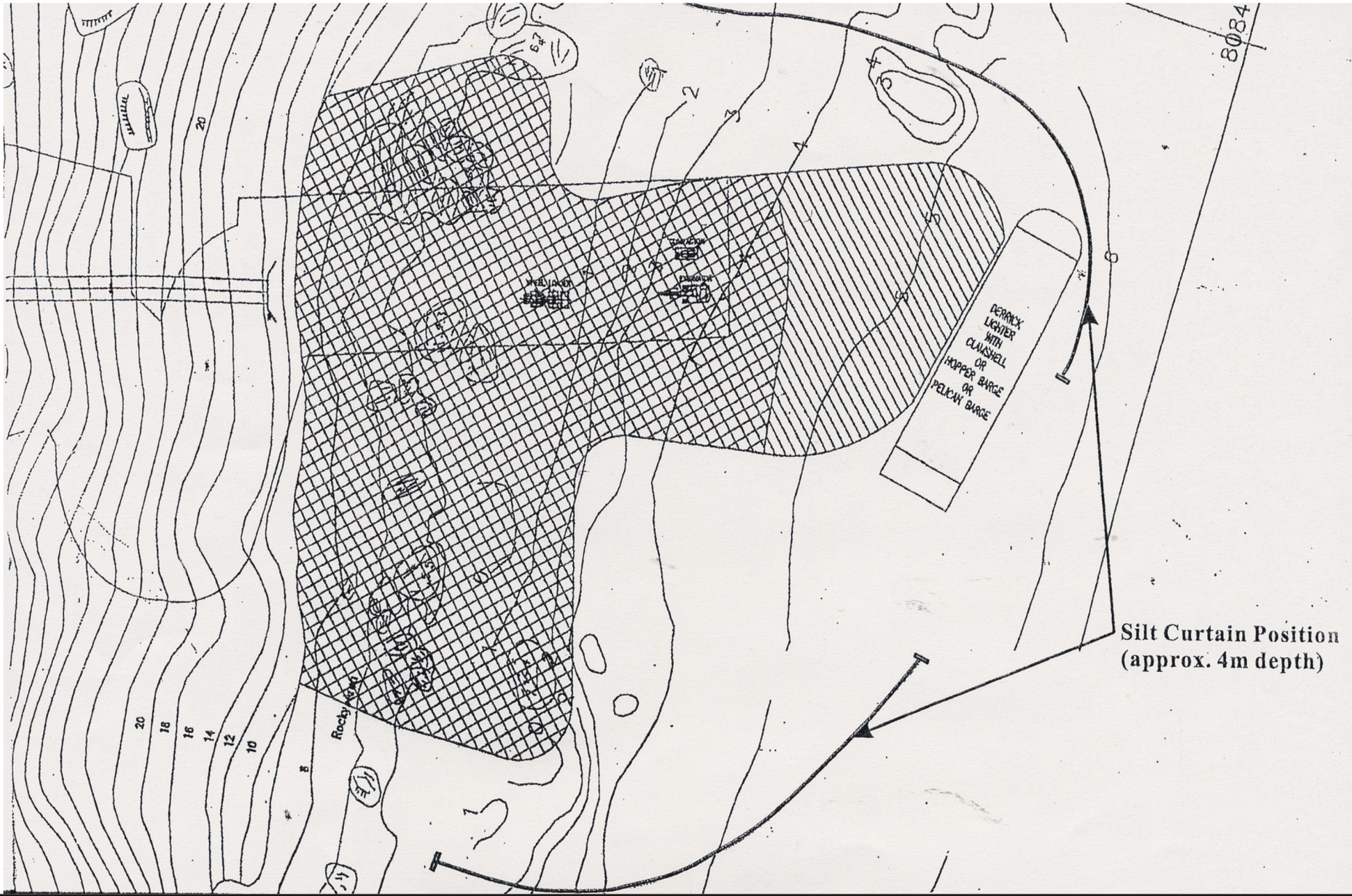
Location of Silt Curtain Installation at Tai Long Wan
