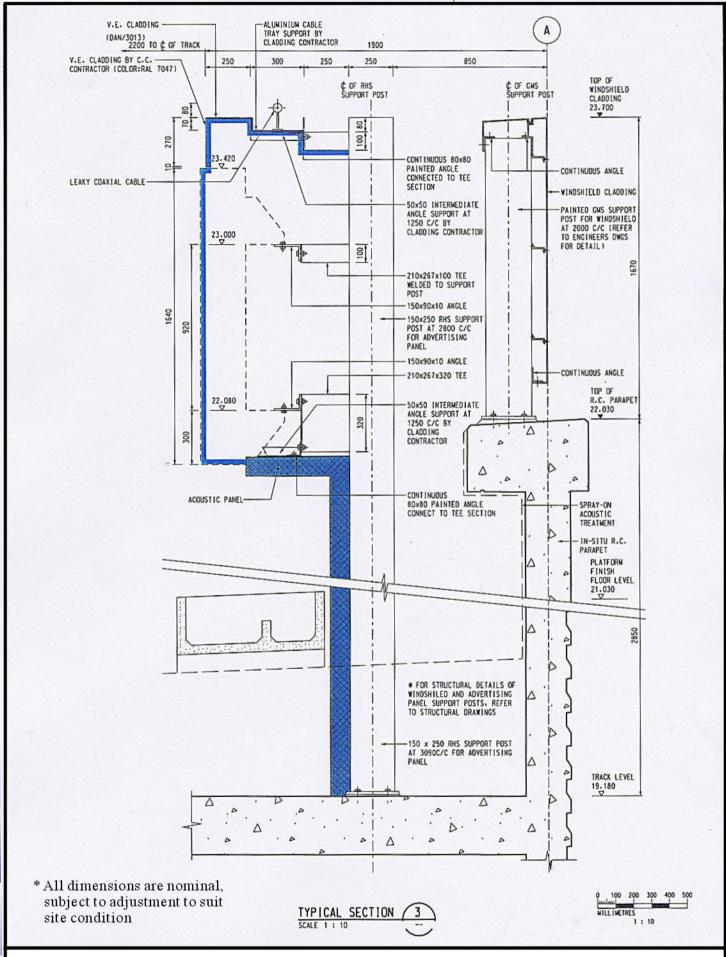
Figure 5 - Trackside Panels and Windshields at the Yuen Long Station [Uptrack (track from Kowloon to Tuen Mun)]
