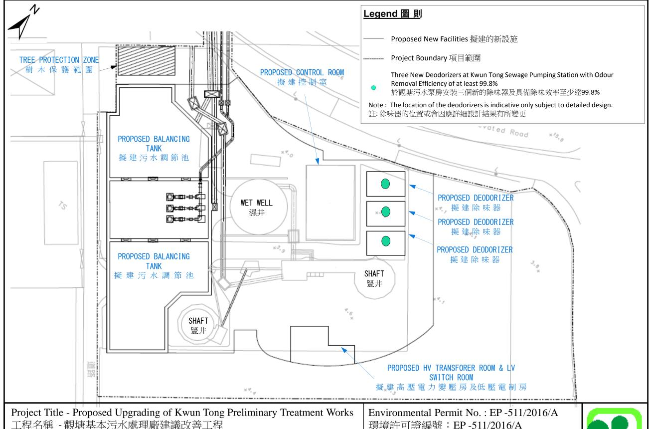
Figure 3 - Layout of the Existing Kwun Tong Sewage Pumping Station and Proposed Balancing Tank and Location of Deodorizers
