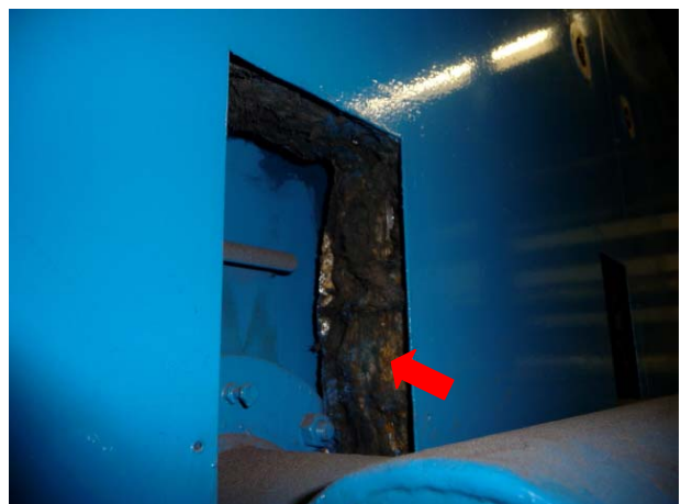
Photo 12. Glass fibre insulation of the incinerator, photo taken at Incinerator 2.
