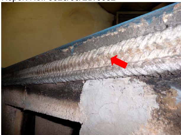
Photo 13. Nylon Insulation of the Incinerator Door, photo taken at Incinerator 1.
