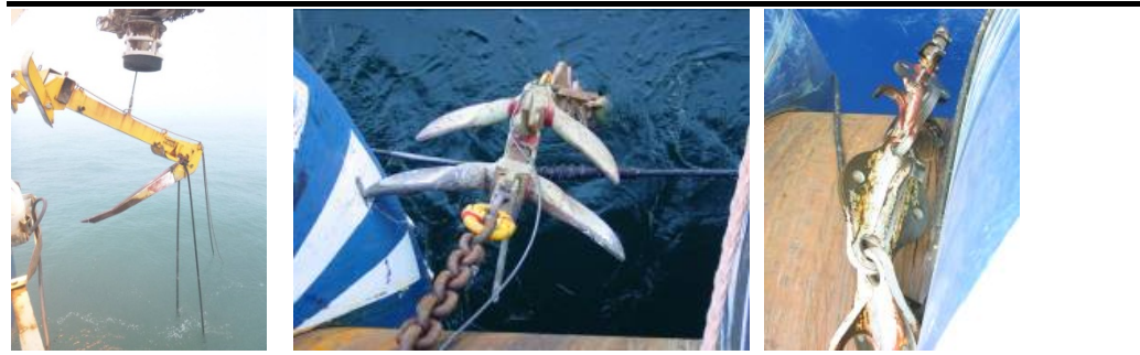
Figure 2.17 Typical grapnels used to penetrate seabed, grip, cut and recover cable
