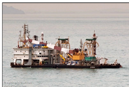
Typical Cable Installation Barge/ Vessel using Injector Burial Tool
