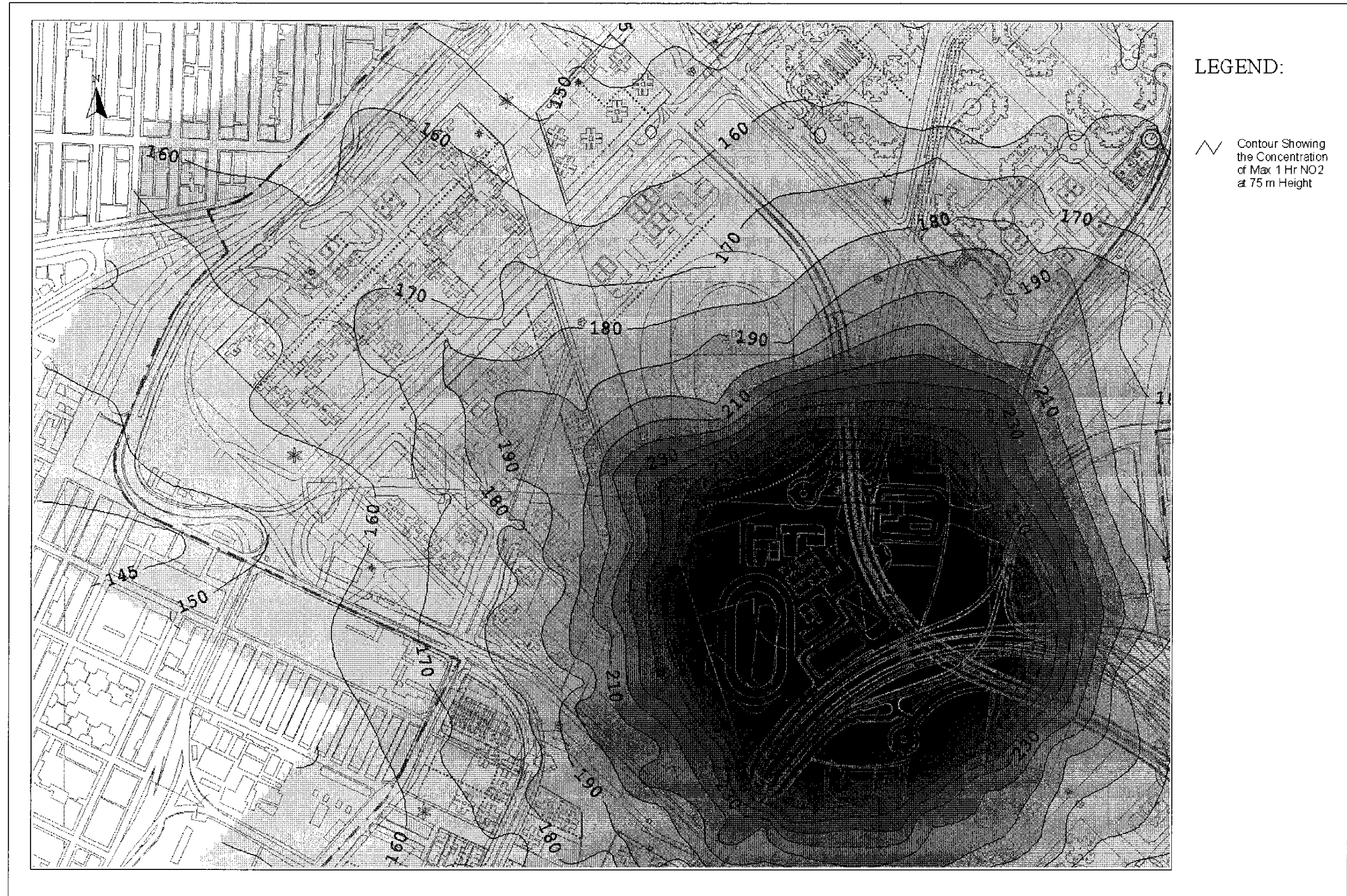
Drawing No. 22936/EN/320B Predicted Worst-case 1-hr Average NO 2 Concentration Contours at 75m Above Ground
