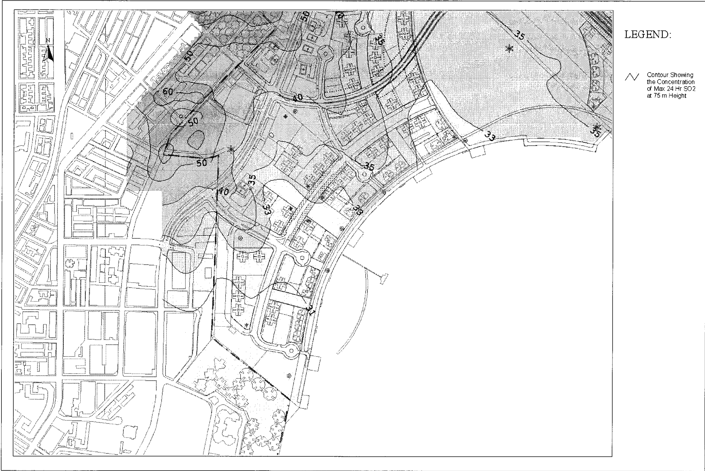
Drawing No. 22936/EN/335D Predicted Worst-case 24-hr Average SO 2 Concentration Contours at 75m Above Ground
