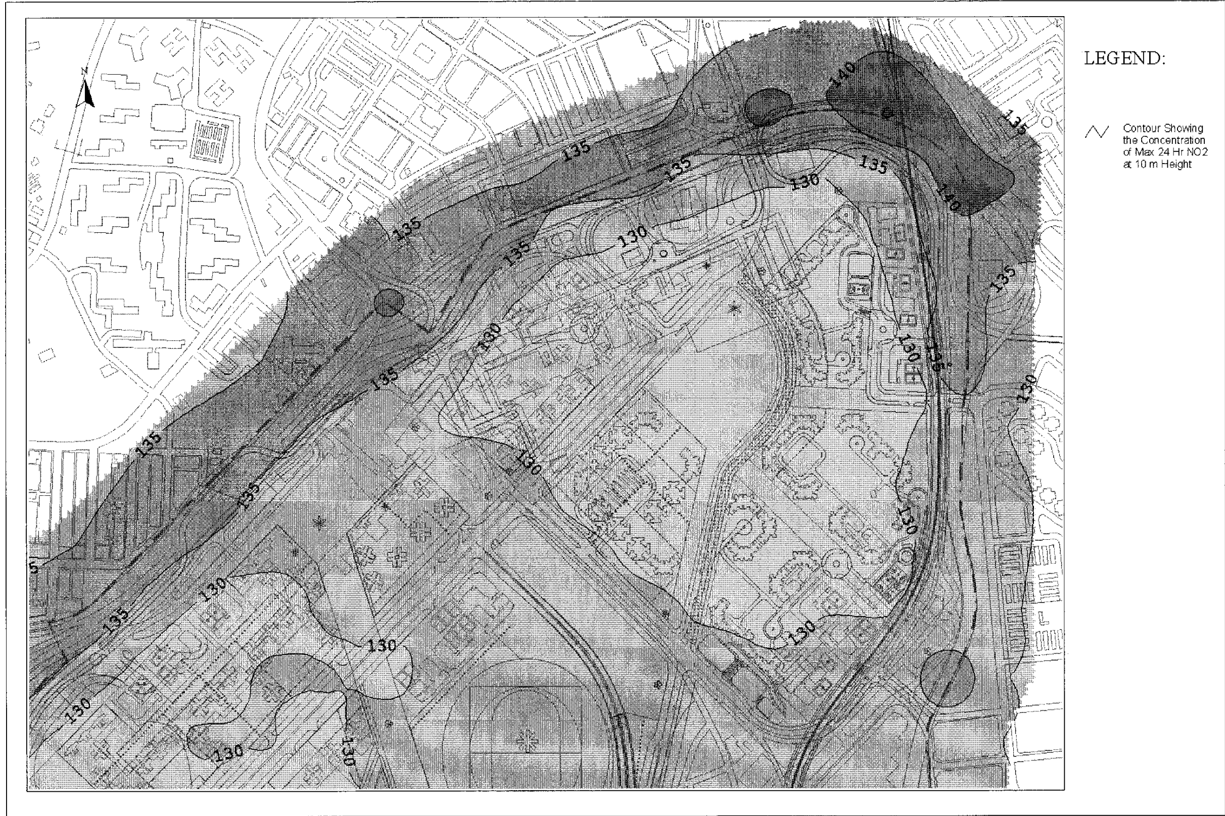
Drawing No. 22936/EN/323A Predicted Worst-case 24-hr Average NO 2 Concentration Contours at 10m Above Ground
