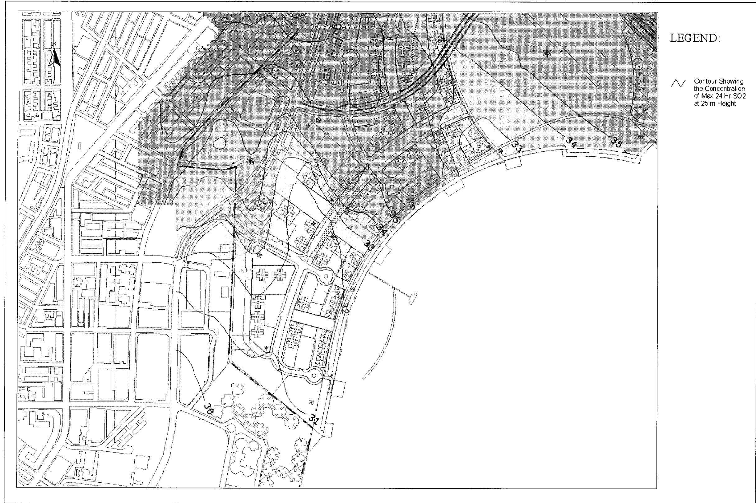
Drawing No. 22936/EN/333D Predicted Worst-case 24-hr Average SO 2 Concentration Contours at 25m Above Ground
