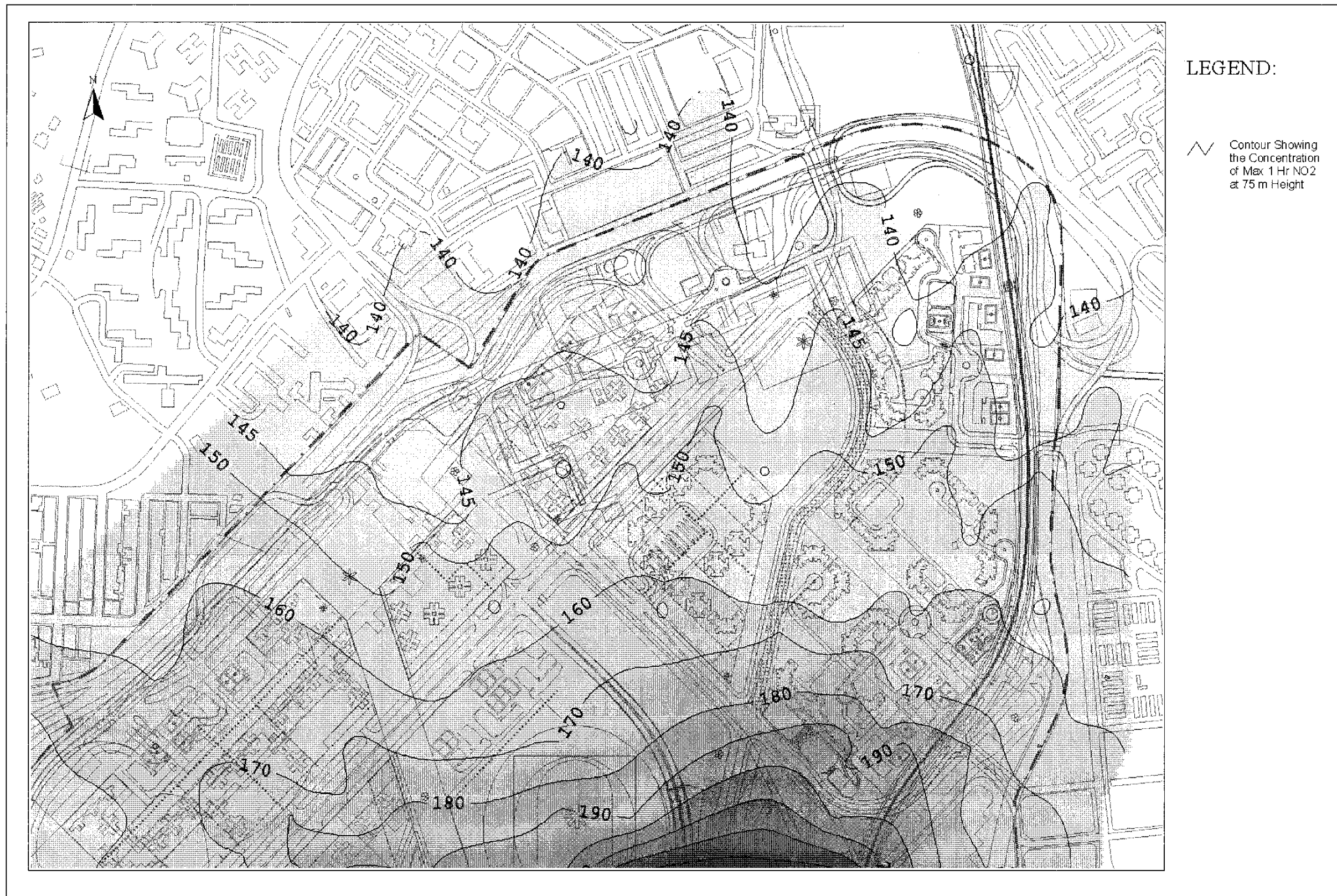
Drawing No. 22936/EN/320A Predicted Worst-case 1-hr Average NO 2 Concentration Contours at 75m Above Ground
