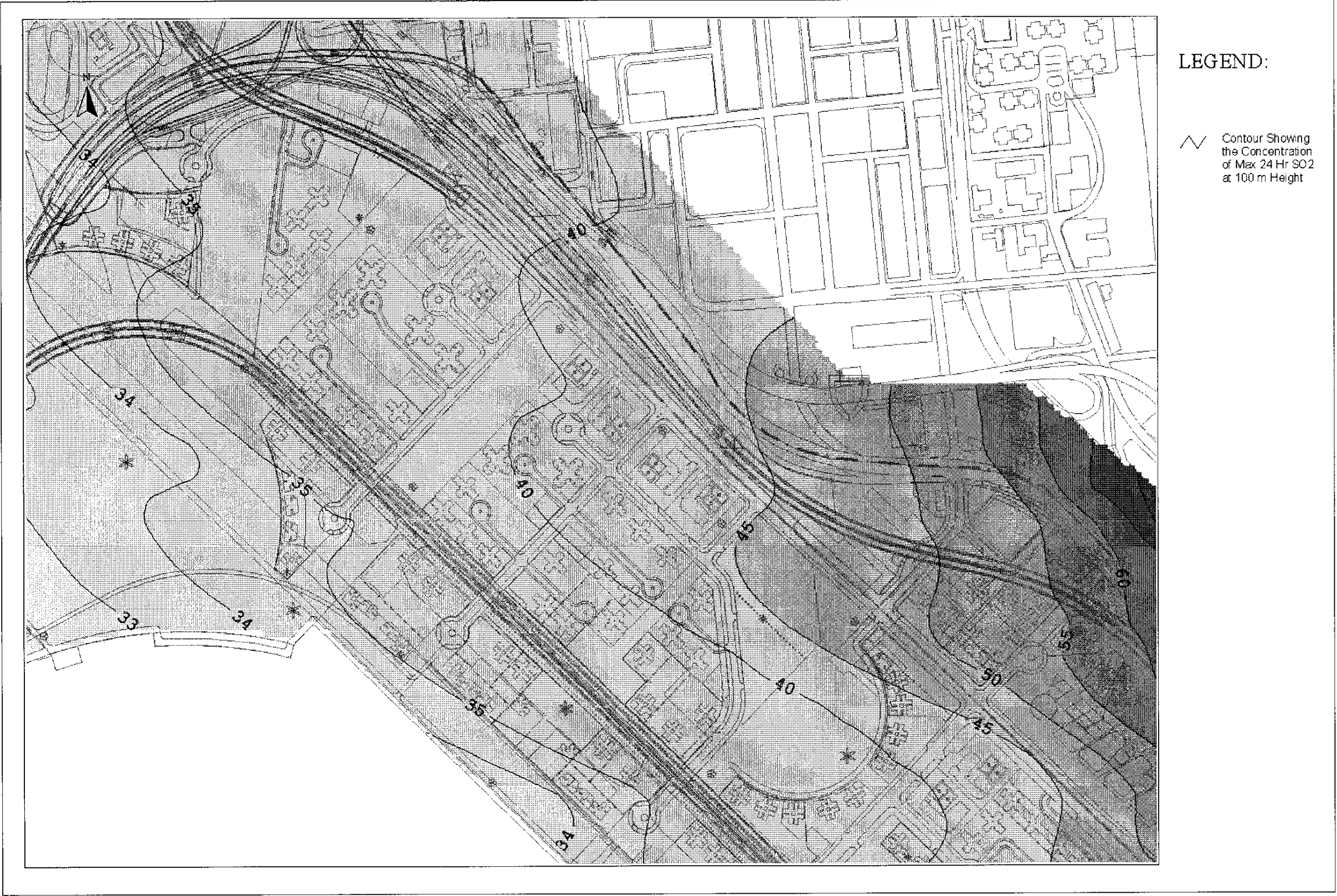
Drawing No. 22936/EN/336E Predicted Worst-case 24-hr Average SO 2 Concentration Contours at 100m Above Ground
