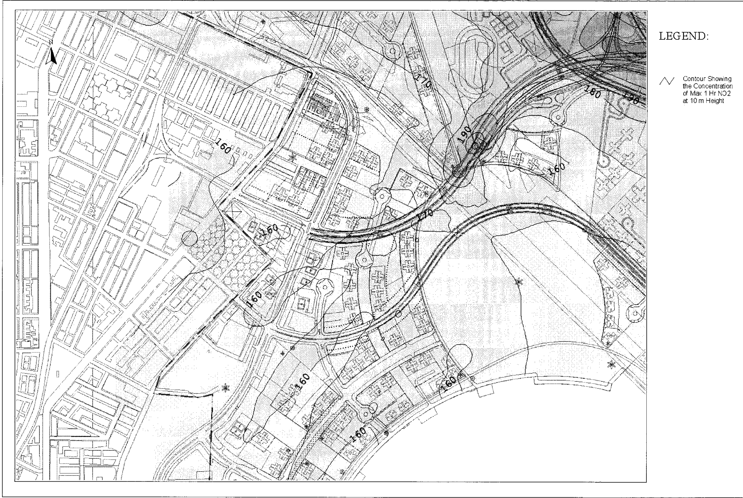
Drawing No. 22936/EN/317C Predicted Worst-case 1-hr Average NO 2 Concentration Contours at 10m Above Ground
