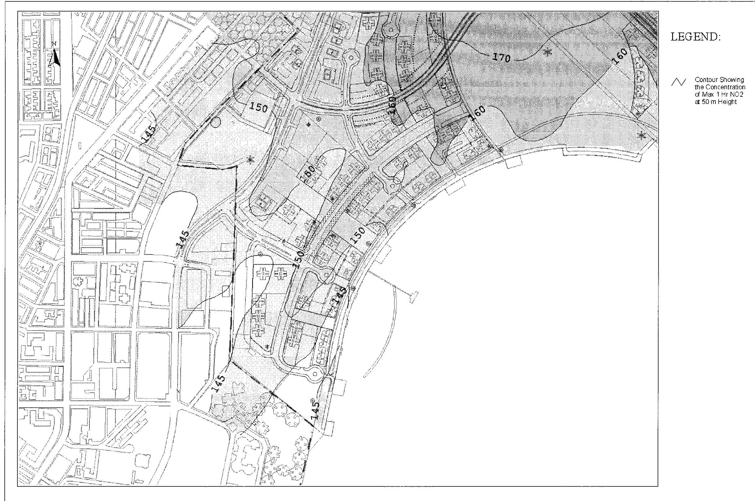
Drawing No. 22936/EN/319D Predicted Worst-case 1-hr Average NO 2 Concentration Contours at 50m Above Ground
