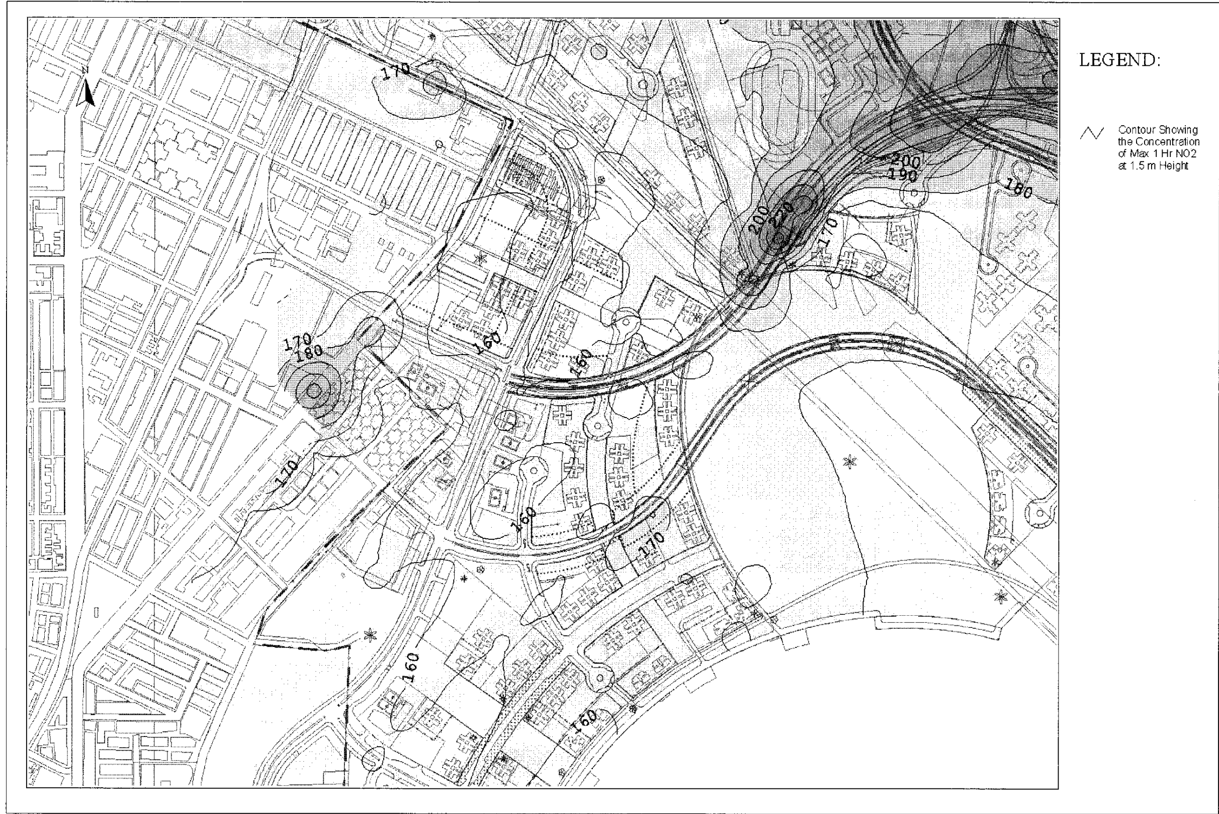
Drawing No. 22936/EN/316C Predicted Worst-case 1-hr Average NO 2 Concentration Contours at 1.5m Above Ground
