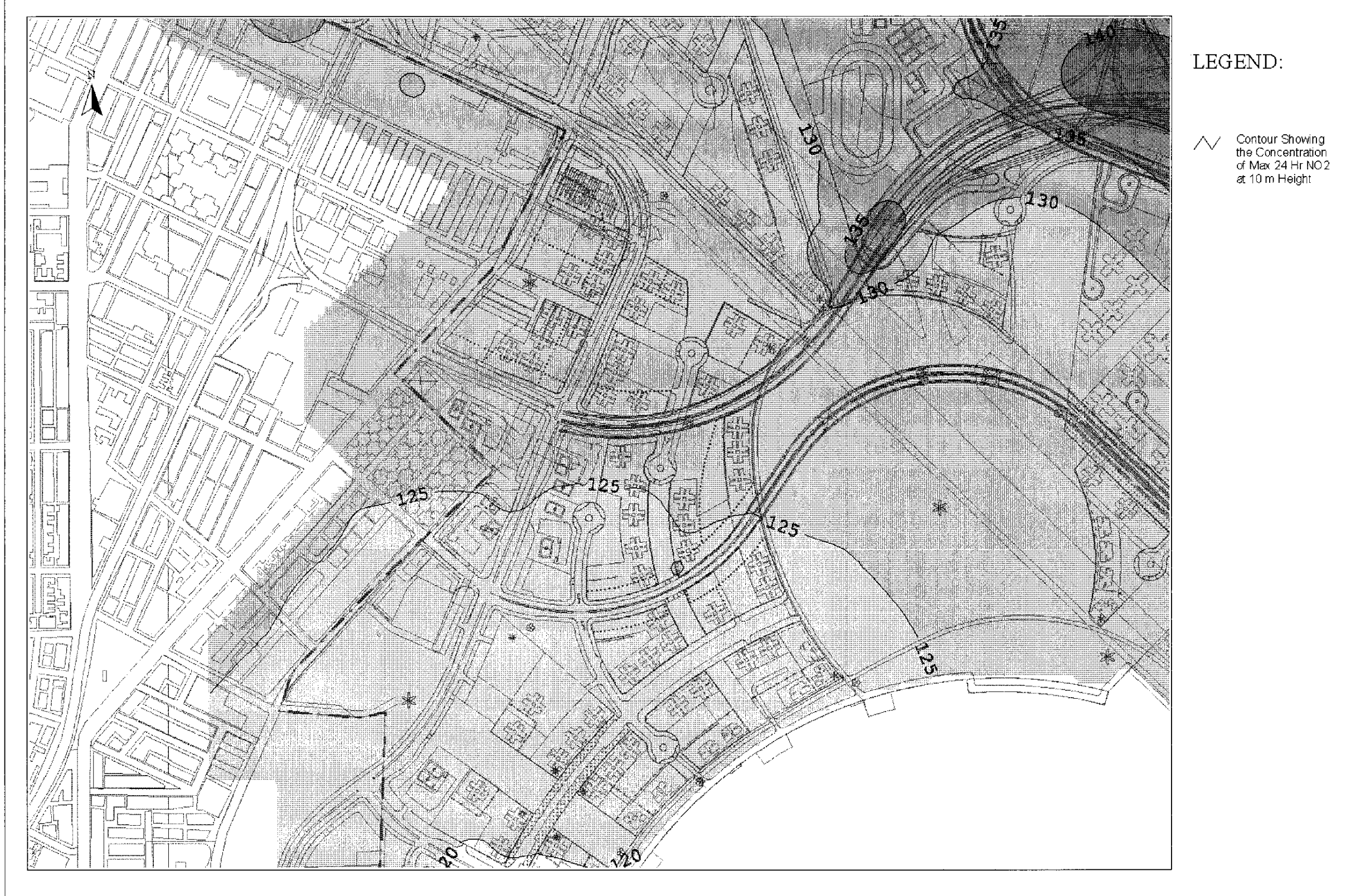
Drawing No. 22936/EN/323C Predicted Worst-case 24-hr Average NO 2 Concentration Contours at 10m Above Ground
