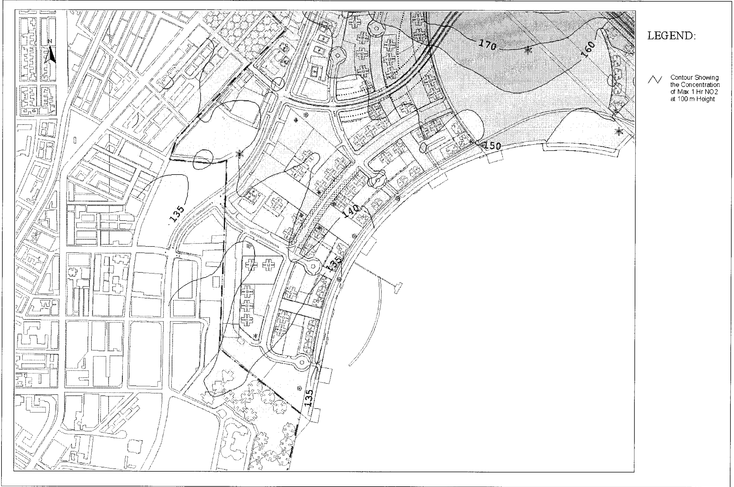
Drawing No. 22936/EN/321D Predicted Worst-case 1-hr Average NO 2 Concentration Contours at 100m Above Ground
