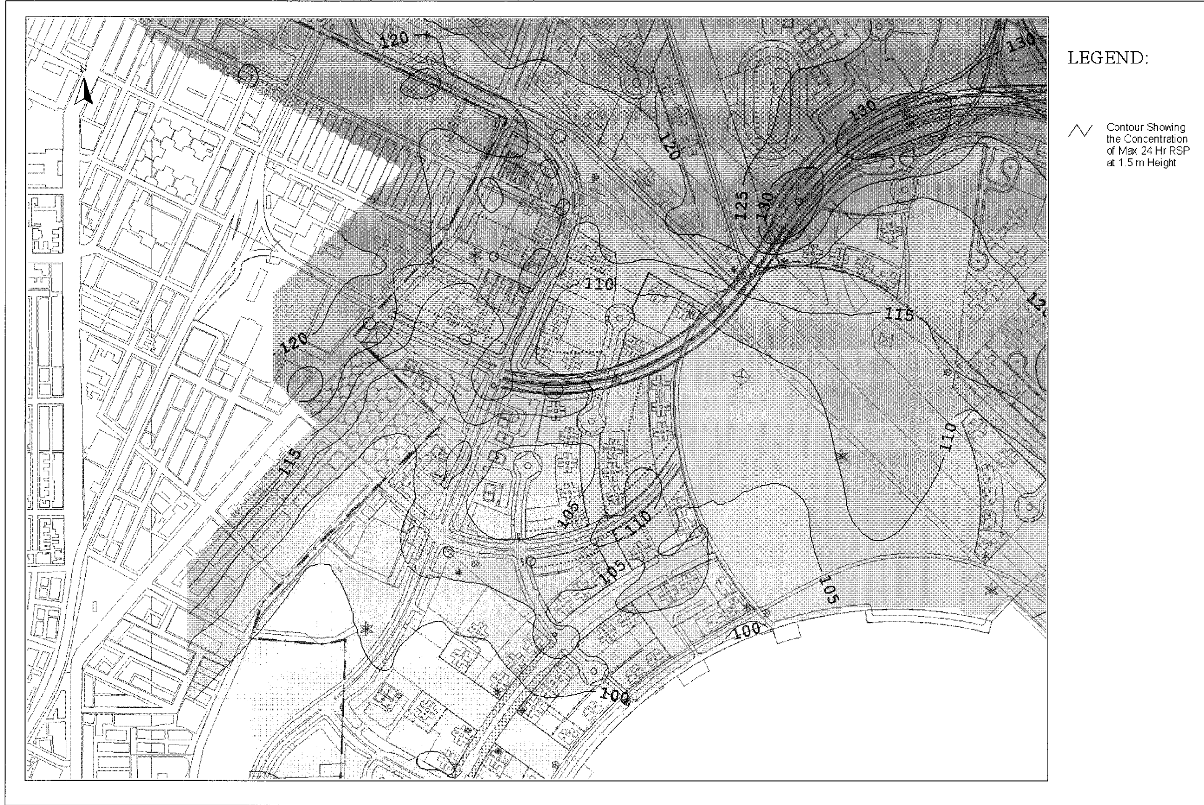
Drawing No. 22936/EN/328C Predicted Worst-case 24-hr Average RSP Concentration Contours at 1.5m Above Ground
