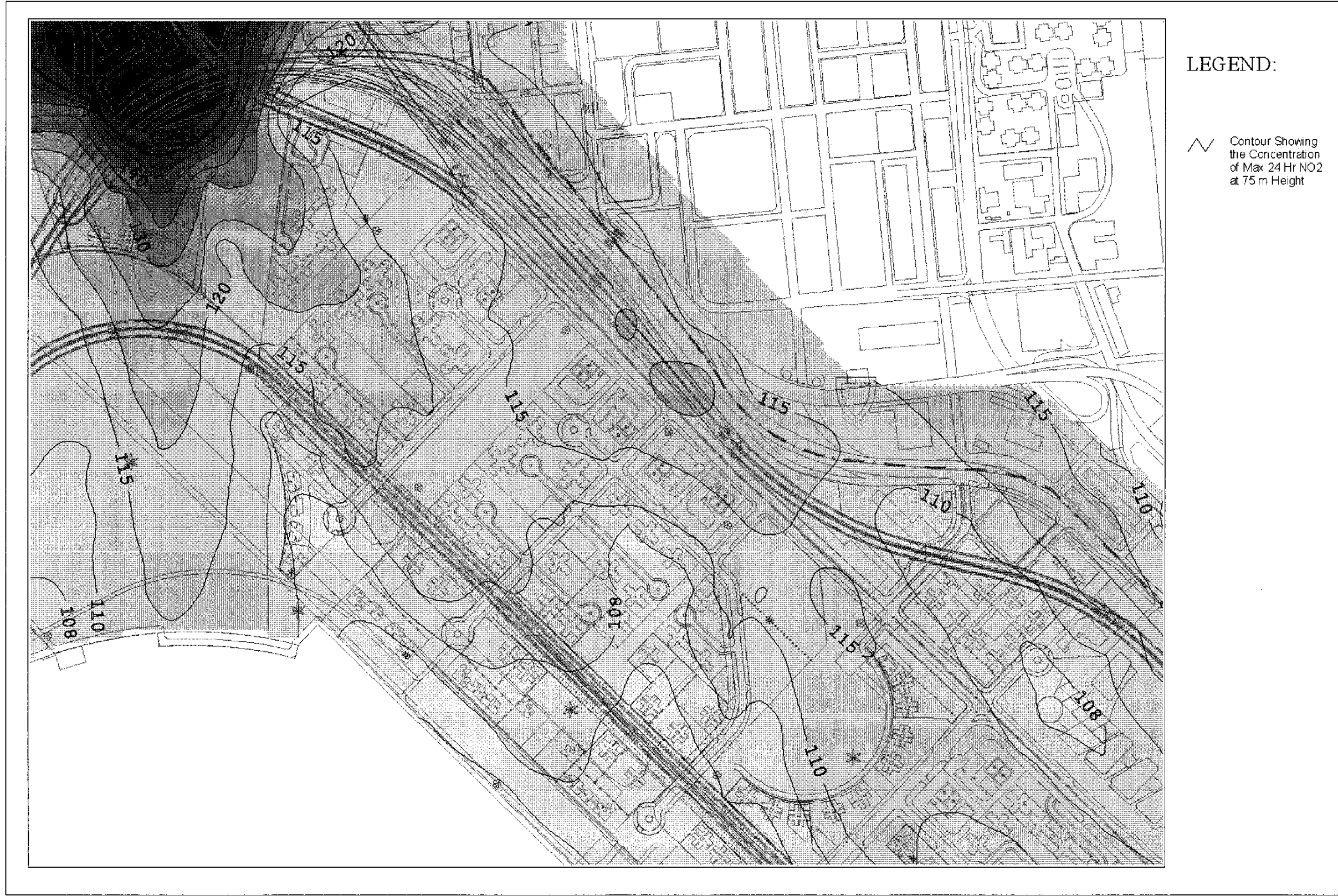
Drawing No. 22936/EN/326E Predicted Worst-case 24-hr Average NO 2 Concentration Contours at 75m Above Ground
