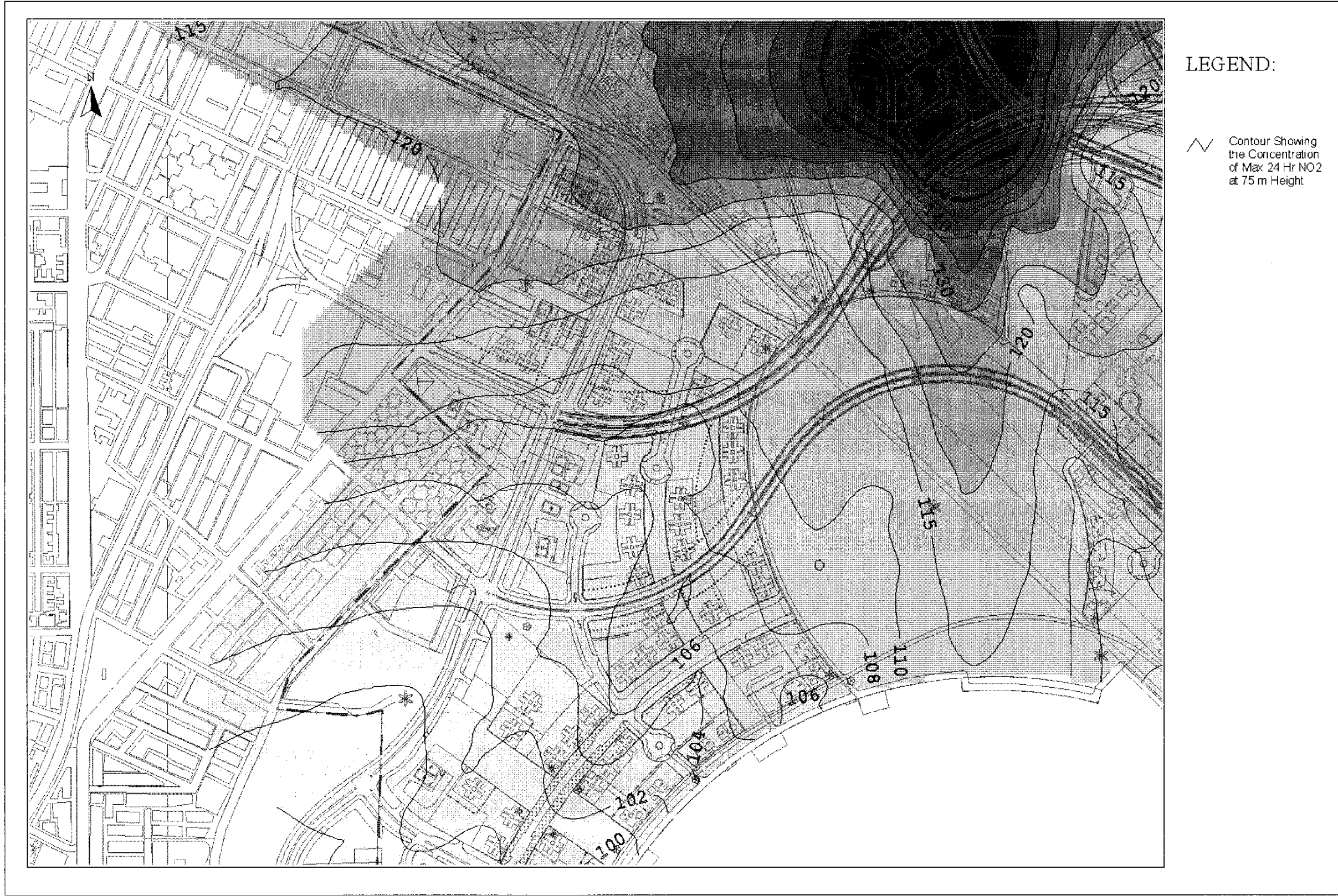
Drawing No. 22936/EN/326C Predicted Worst-case 24-hr Average NO 2 Concentration Contours at 75m Above Ground
