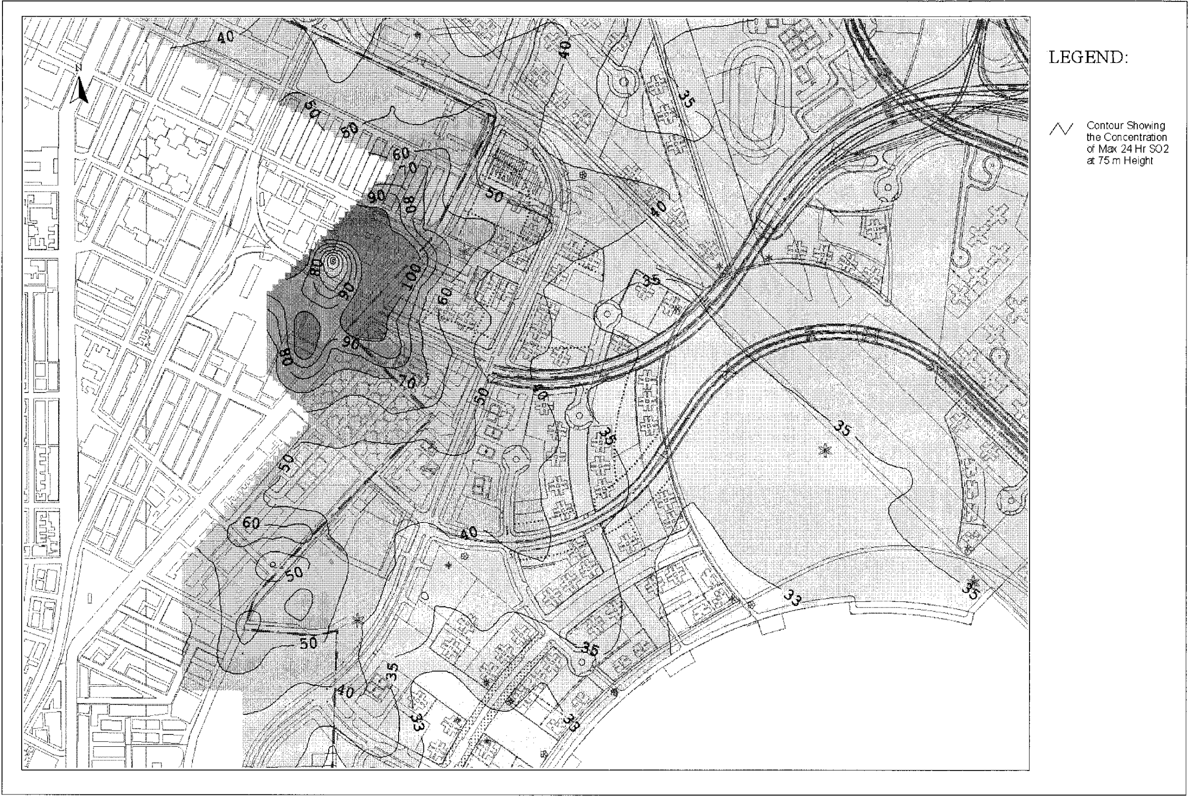
Drawing No. 22936/EN/335C Predicted Worst-case 24-hr Average SO 2 Concentration Contours at 75m Above Ground
