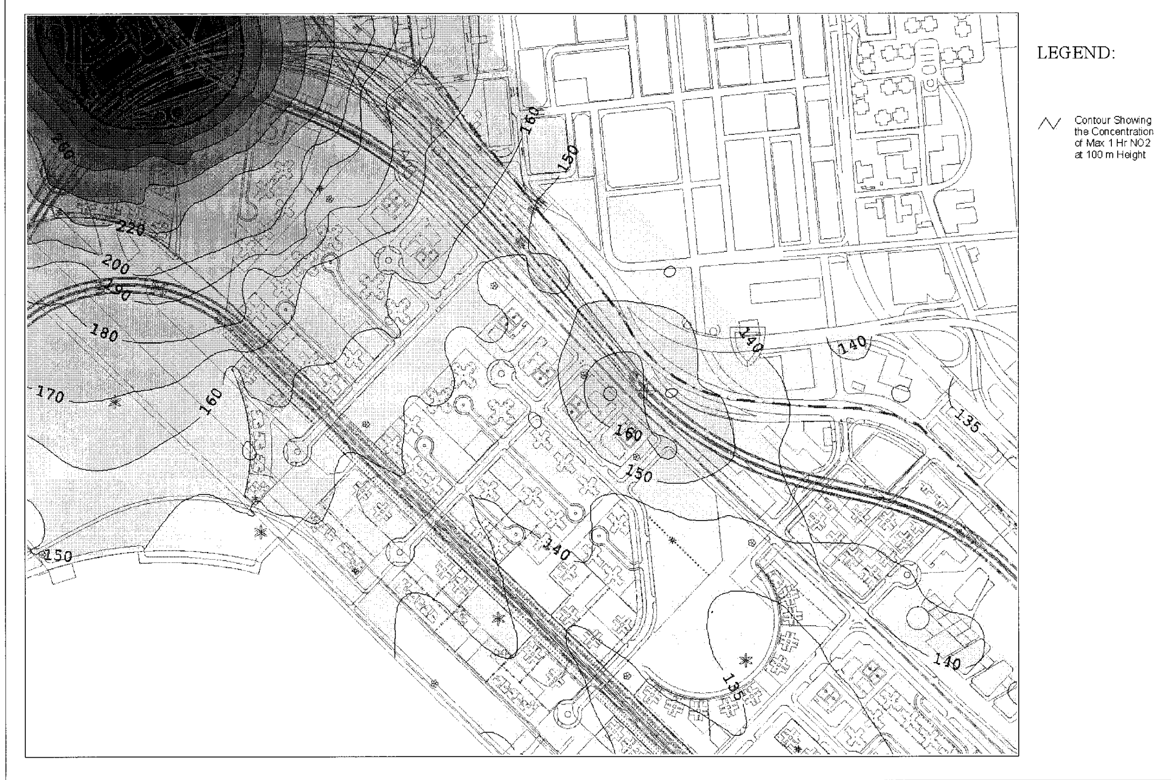
Drawing No. 22936/EN/321E Predicted Worst-case 1-hr Average NO 2 Concentration Contours at 100m Above Ground
