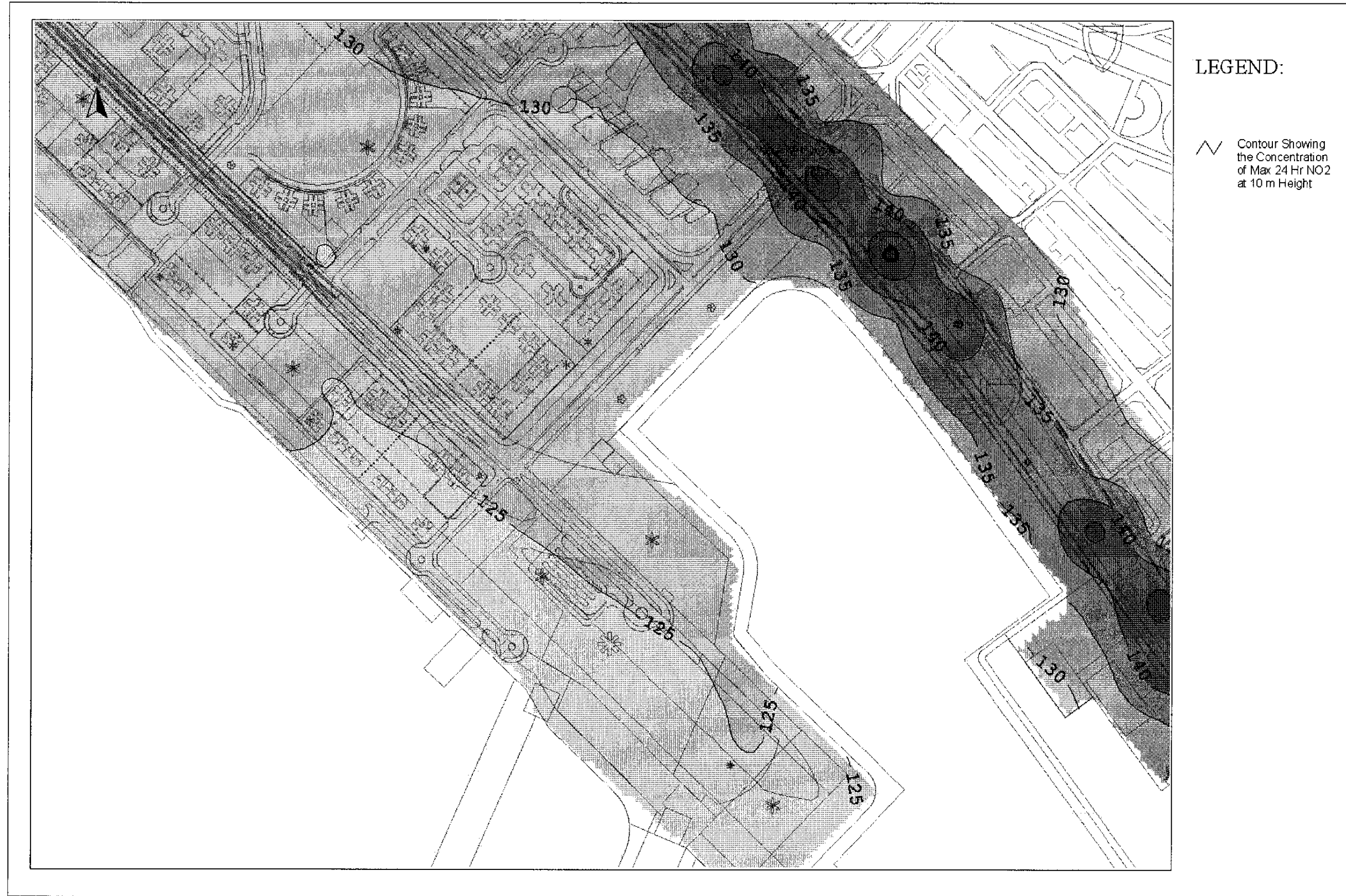
Drawing No. 22936/EN/323F Predicted Worst-case 24-hr Average NO 2 Concentration Contours at 10m Above Ground
