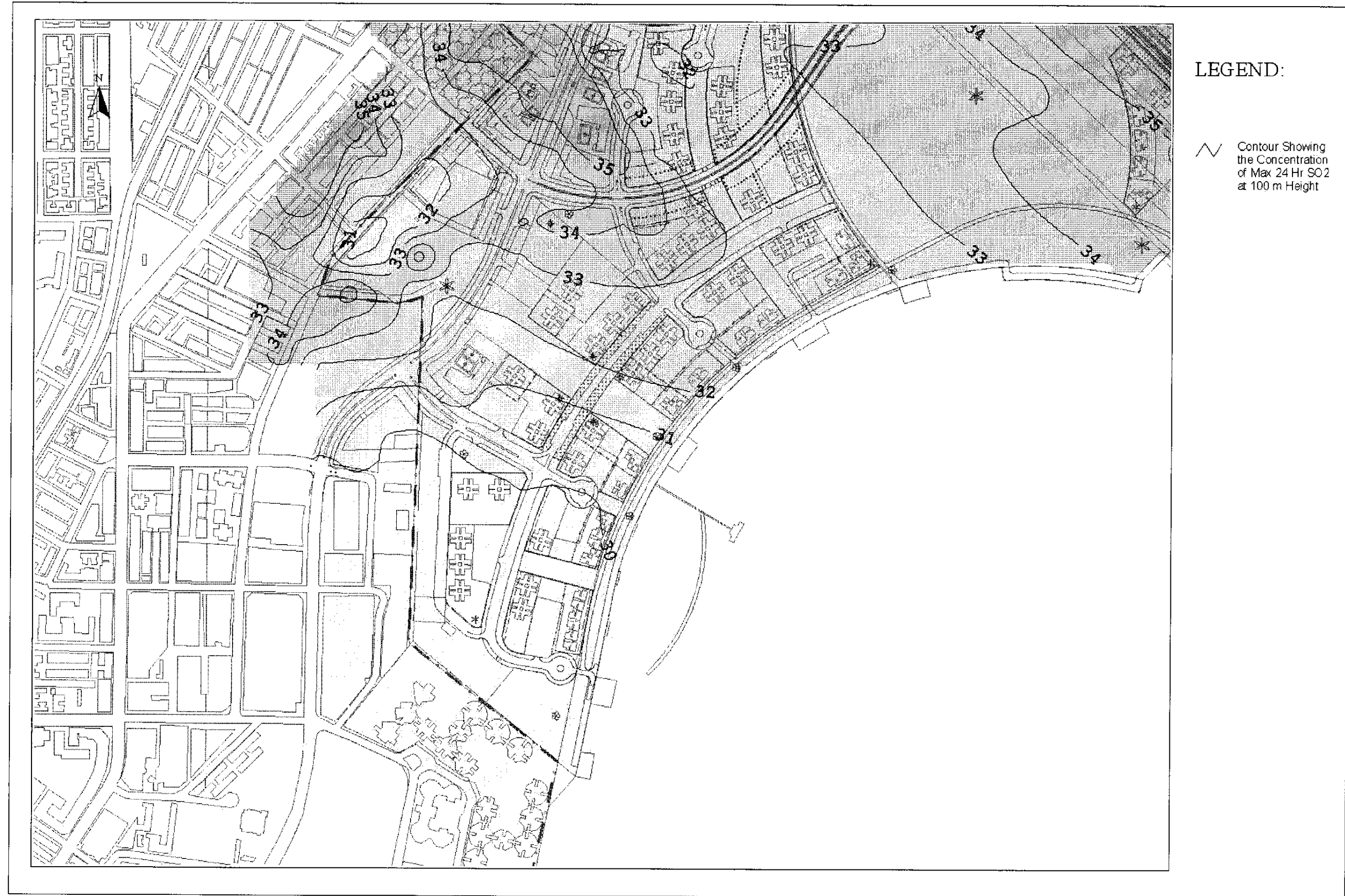
Drawing No. 22936/EN/336D Predicted Worst-case 24-hr Average SO 2 Concentration Contours at 100m Above Ground
