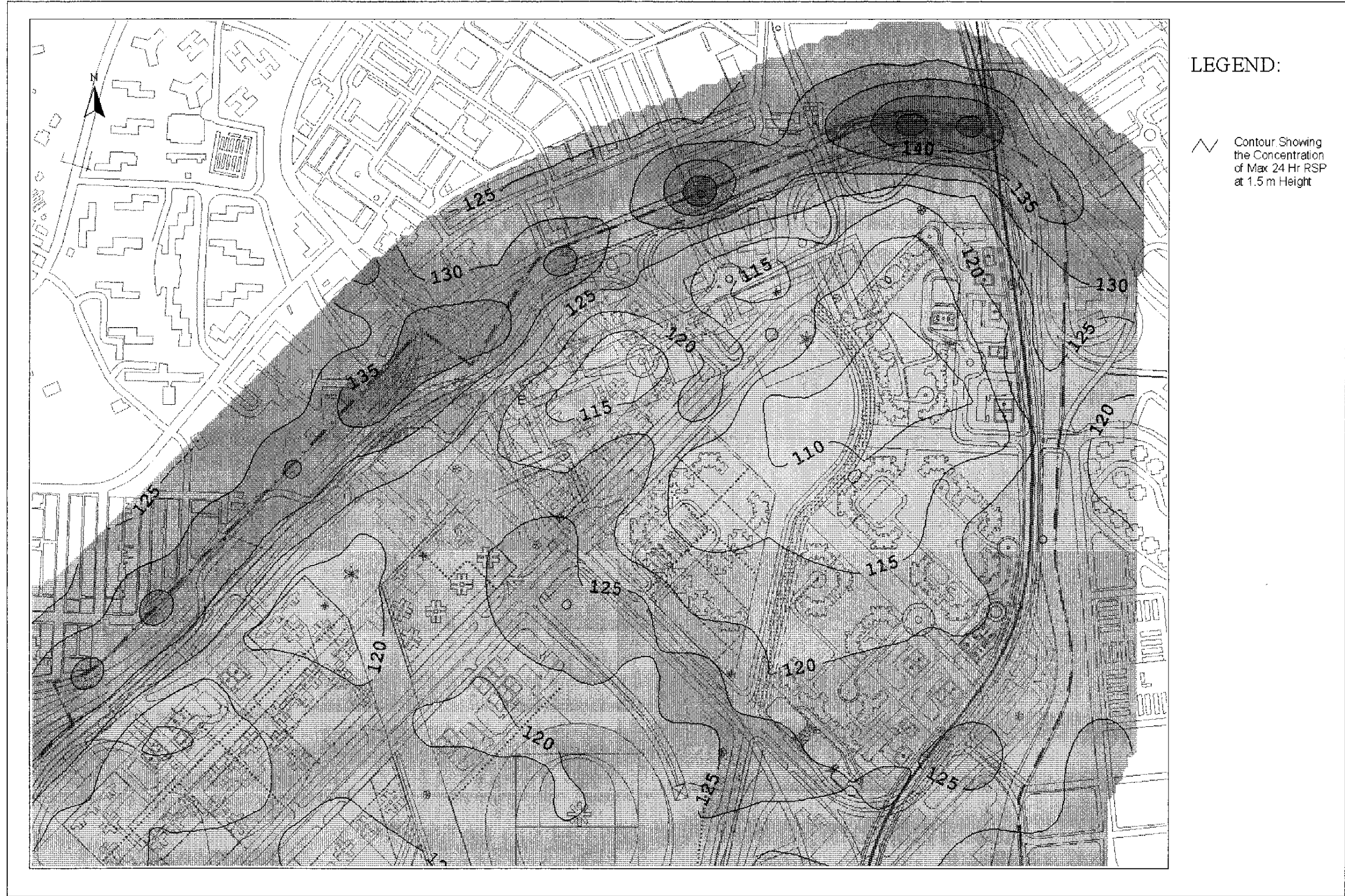
Drawing No. 22936/EN/328A Predicted Worst-case 24-hr Average RSP Concentration Contours at 1.5m Above Ground
