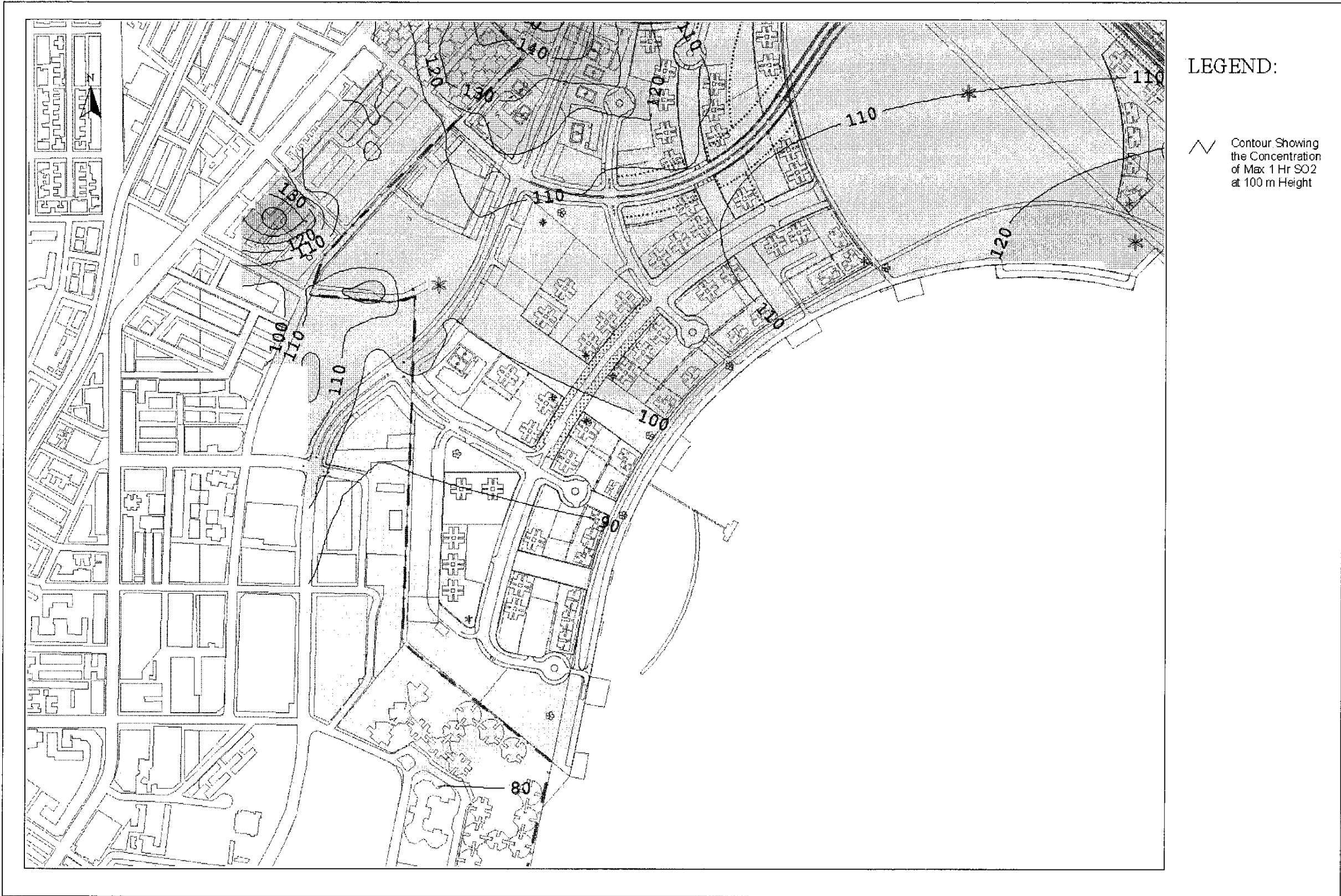
Drawing No. 22936/EN/332D Predicted Worst-case 1-hr Average SO 2 Concentration Contours at 100m Above Ground
