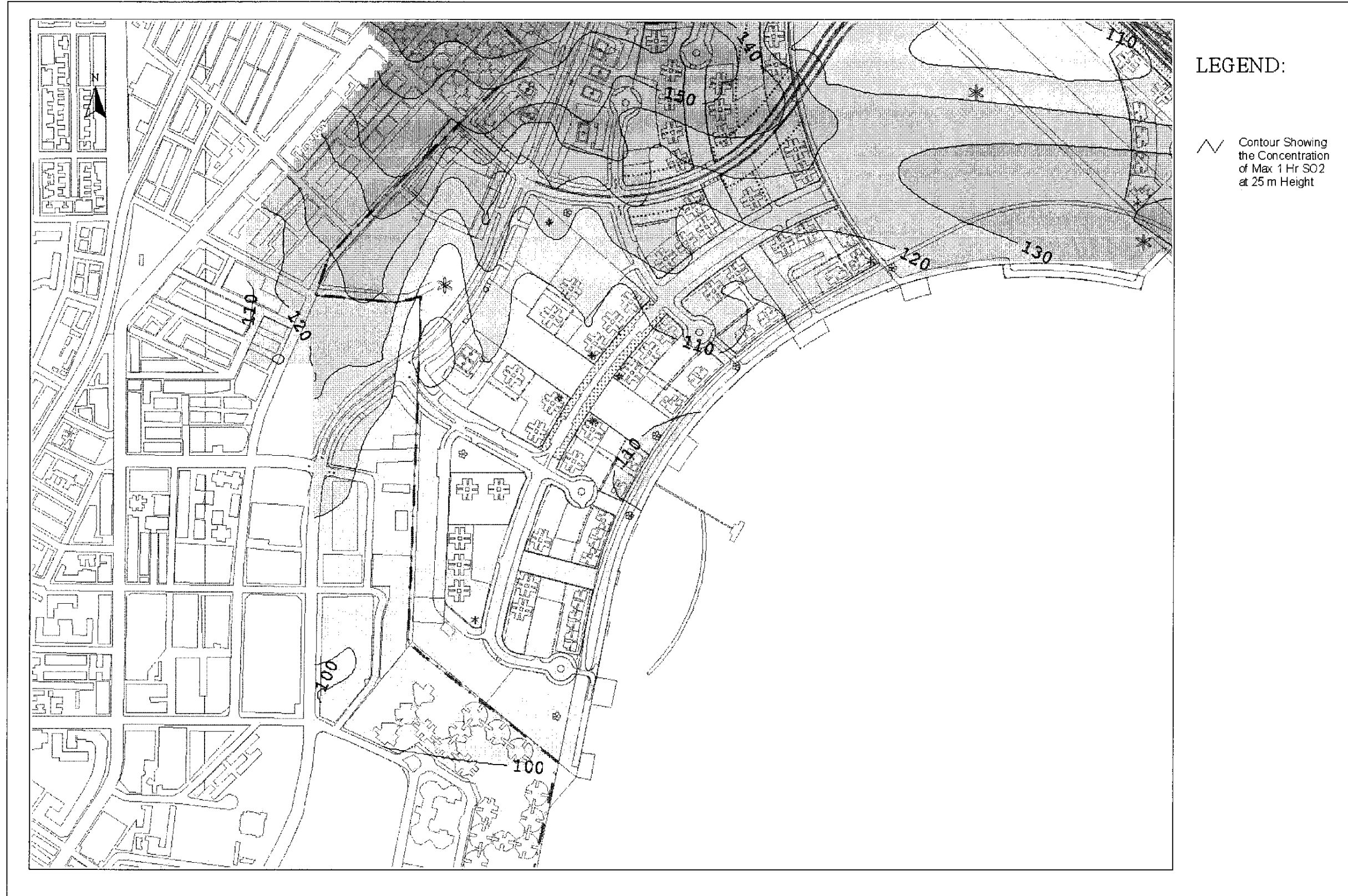
Drawing No. 22936/EN/329D Predicted Worst-case 1-hr Average SO 2 Concentration Contours at 25m Above Ground
