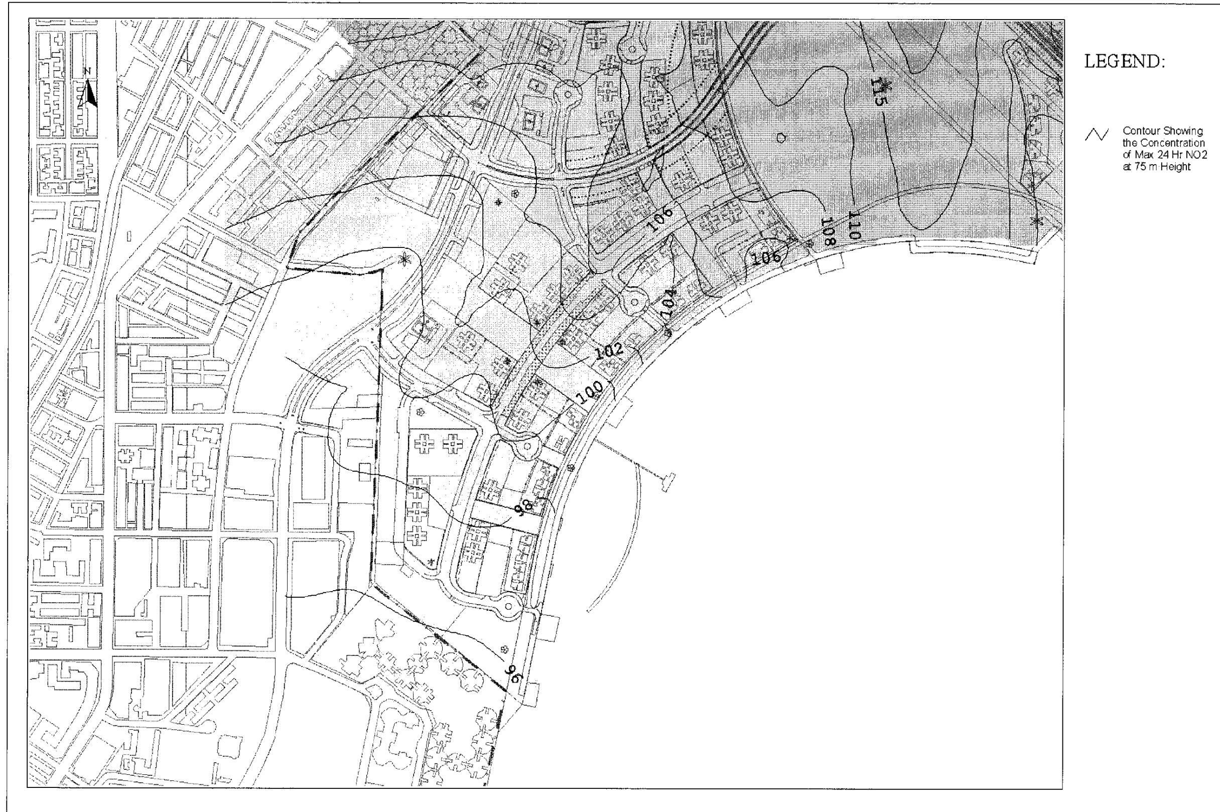
Drawing No. 22936/EN/326D Predicted Worst-case 24-hr Average NO 2 Concentration Contours at 75m Above Ground
