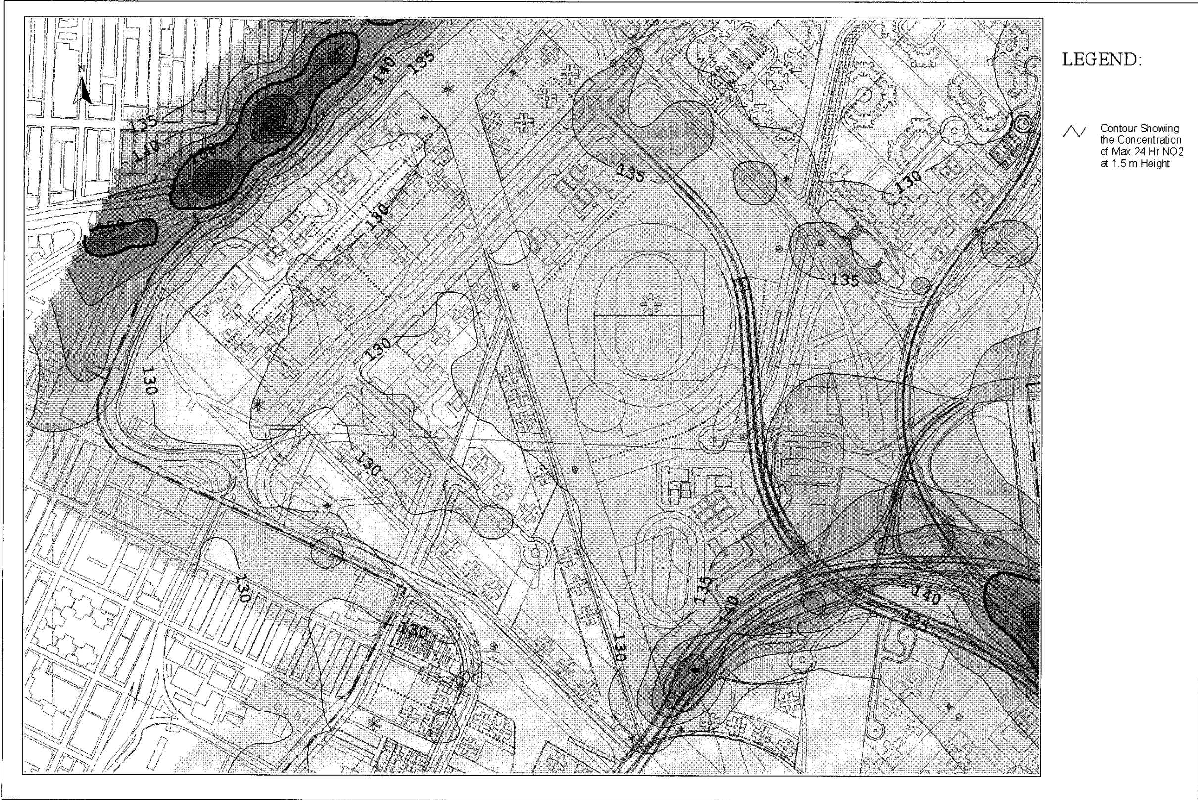
Drawing No. 22936/EN/322B Predicted Worst-case 24-hr Average NO 2 Concentration Contours at 1.5m Above Ground
