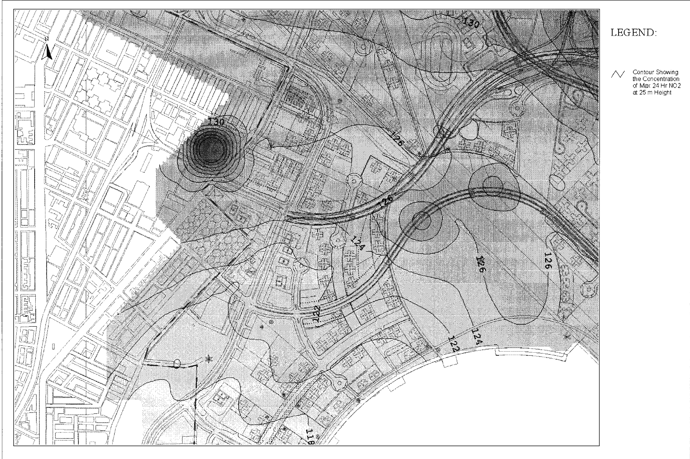
Drawing No. 22936/EN/324C Predicted Worst-case 24-hr Average NO 2 Concentration Contours at 25m Above Ground
