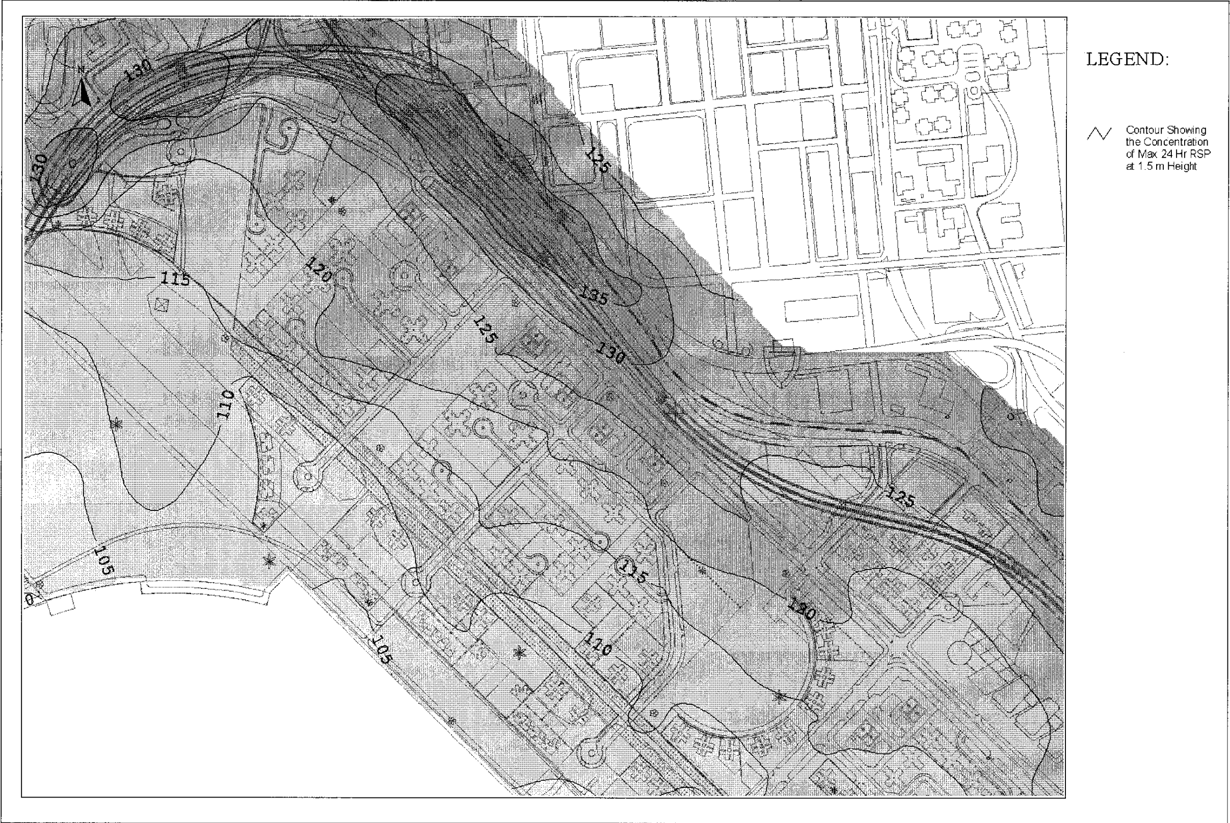
Drawing No. 22936/EN/328E Predicted Worst-case 24-hr Average RSP Concentration Contours at 1.5m Above Ground
