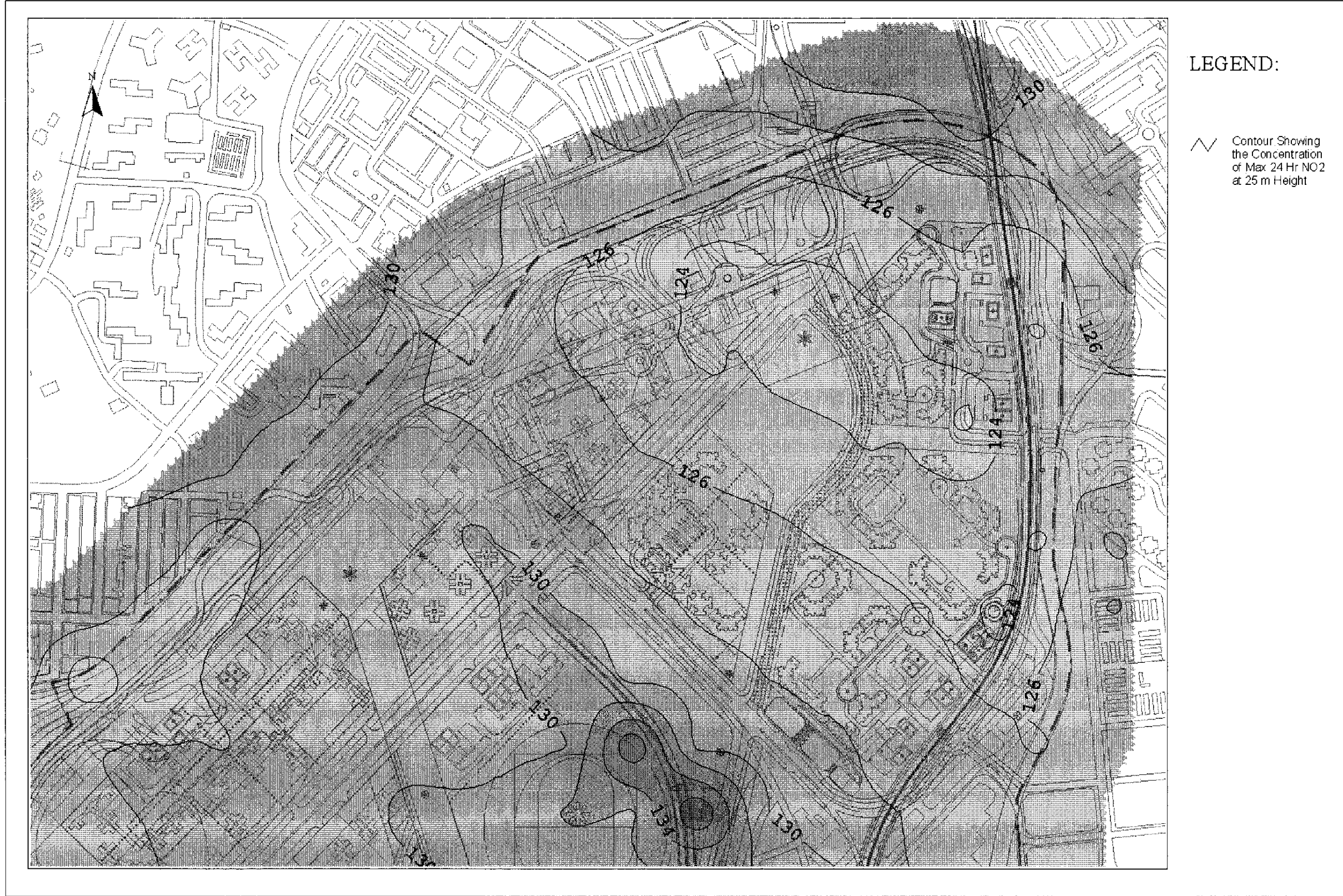
Drawing No. 22936/EN/324A Predicted Worst-case 24-hr Average NO 2 Concentration Contours at 25m Above Ground
