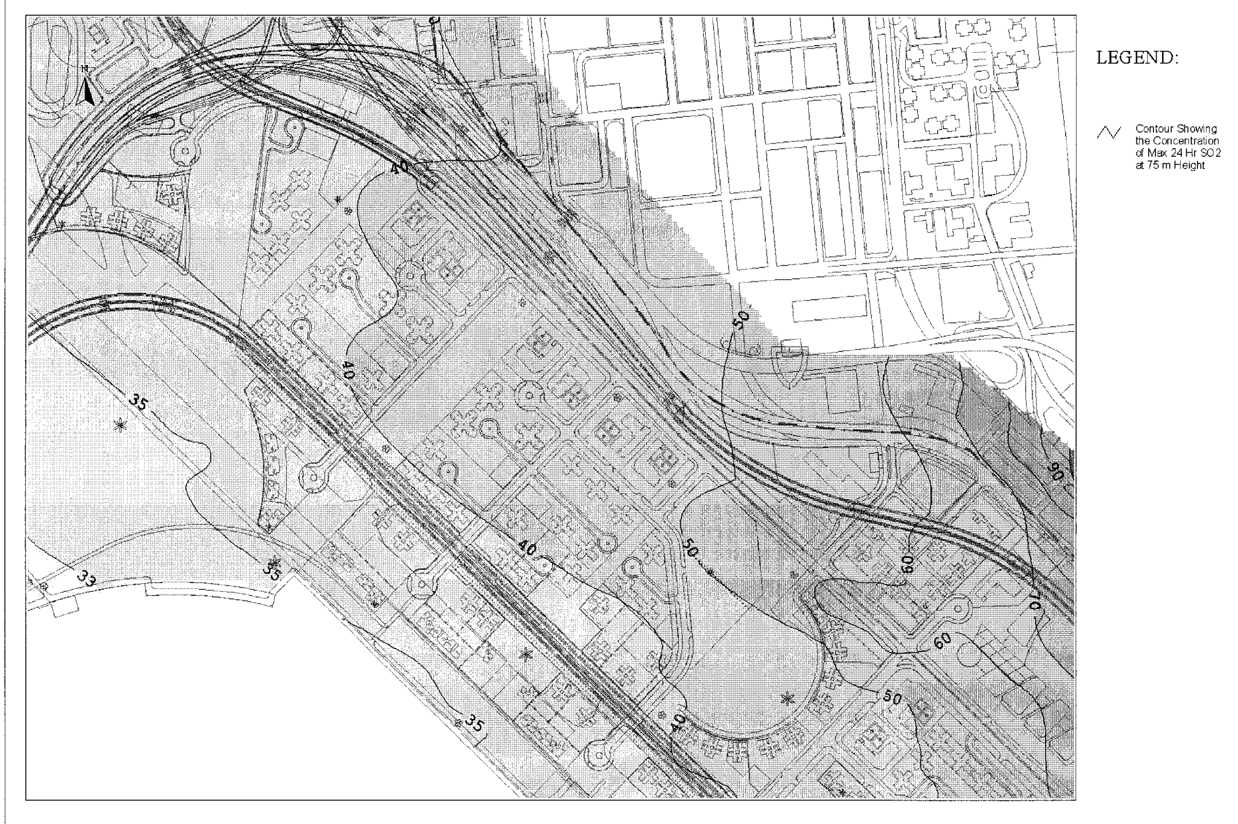
Drawing No. 22936/EN/335E Predicted Worst-case 24-hr Average SO 2 Concentration Contours at 75m Above Ground
