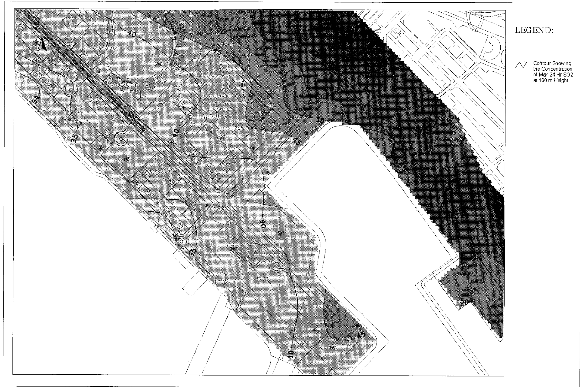
Drawing No. 22936/EN/336F Predicted Worst-case 24-hr Average SO 2 Concentration Contours at 100m Above Ground
