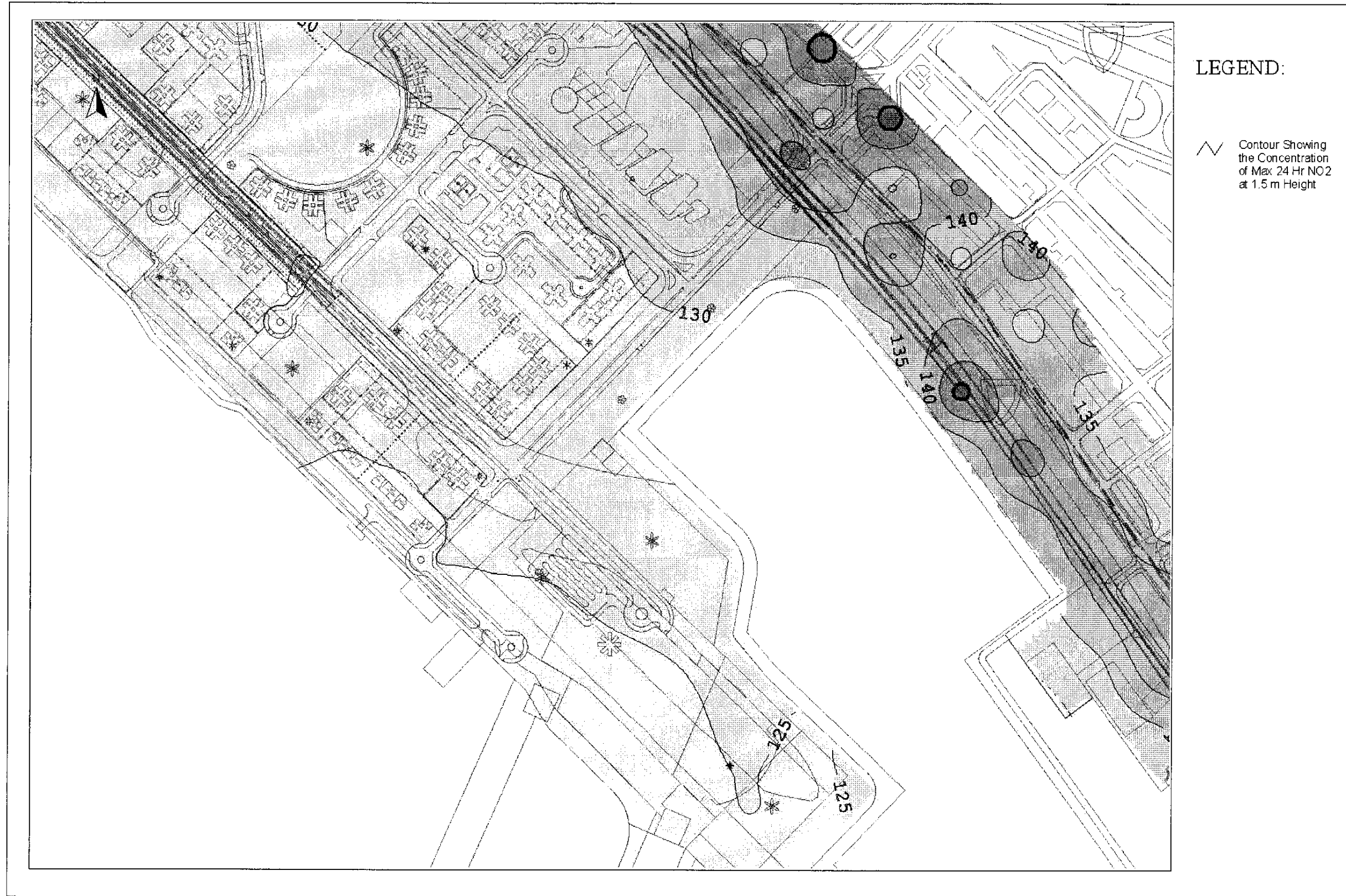
Drawing No. 22936/EN/322F Predicted Worst-case 24-hr Average NO 2 Concentration Contours at 1.5m Above Ground
