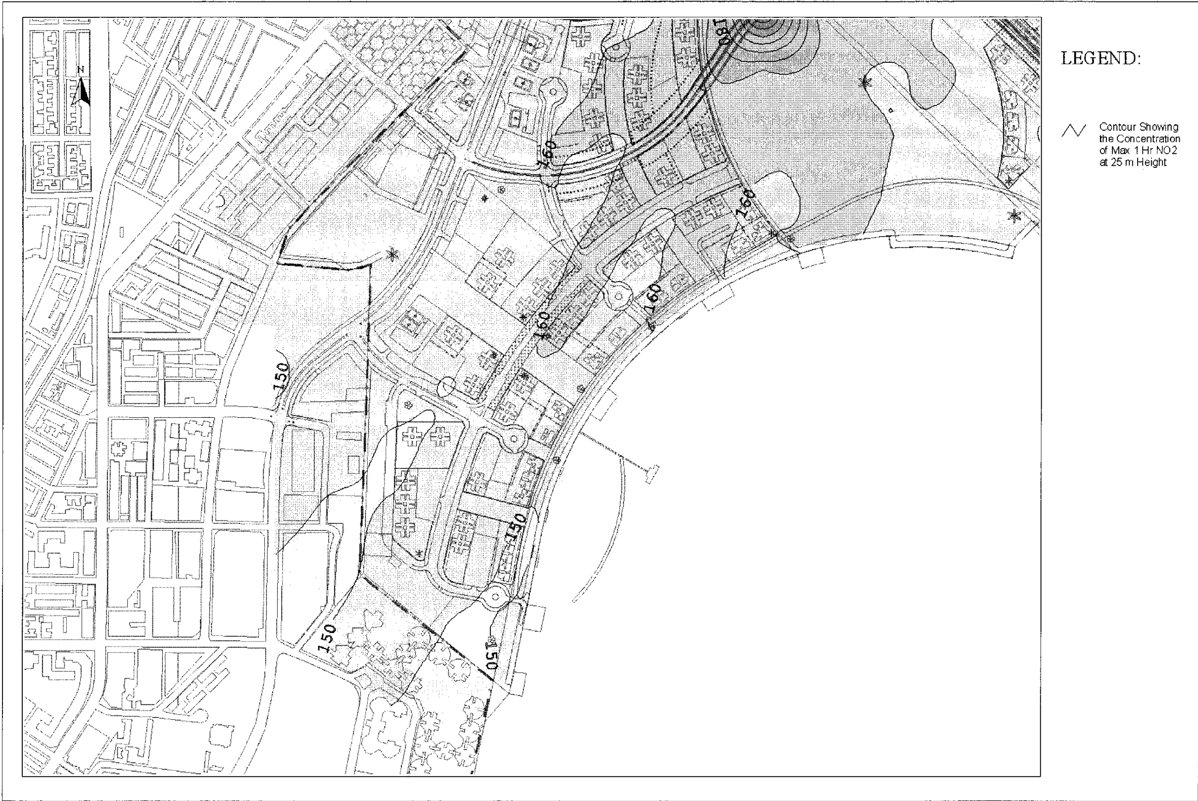
Drawing No. 22936/EN/318D Predicted Worst-case 1-hr Average NO 2 Concentration Contours at 25m Above Ground
