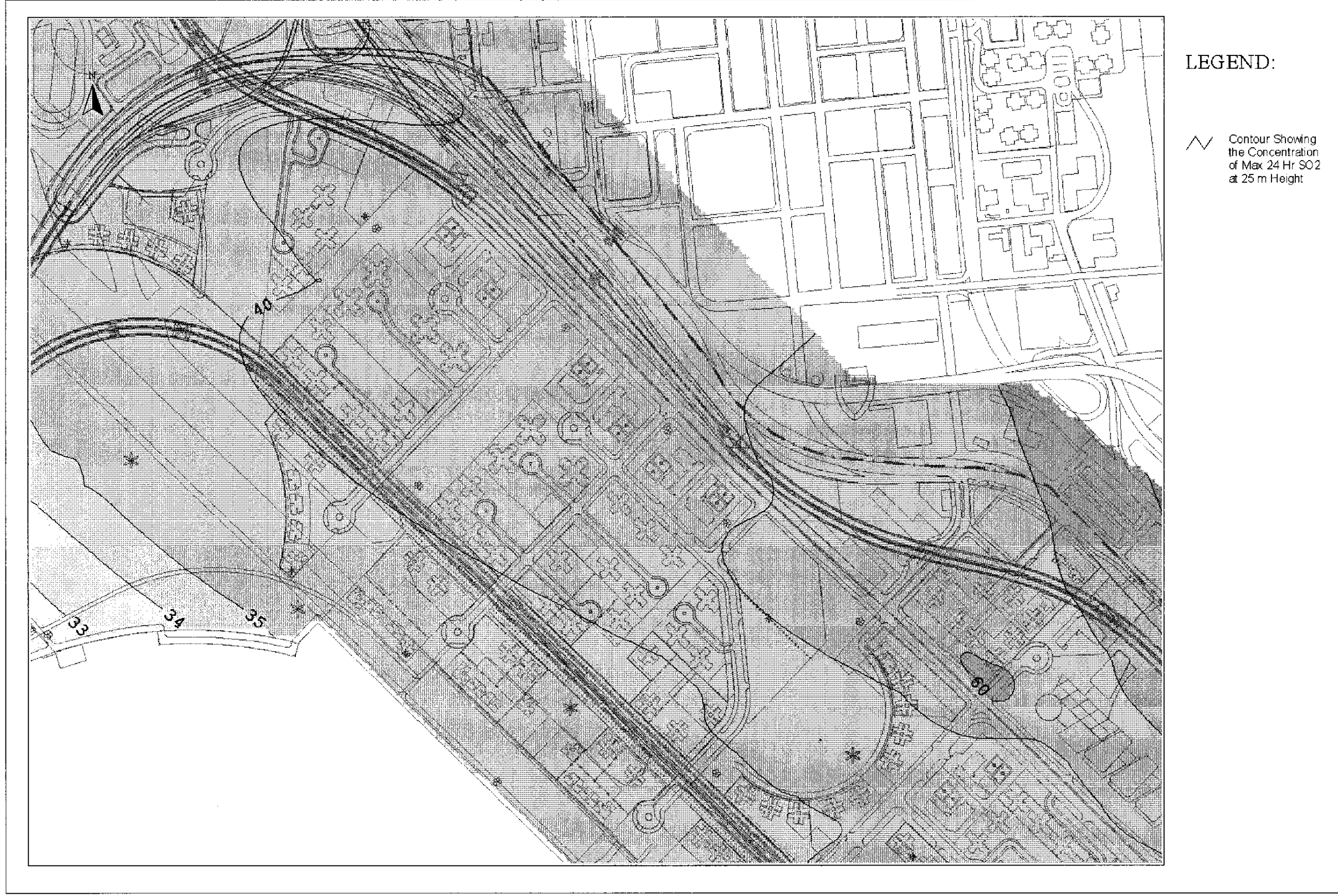
Drawing No. 22936/EN/333E Predicted Worst-case 24-hr Average SO 2 Concentration Contours at 25m Above Ground
