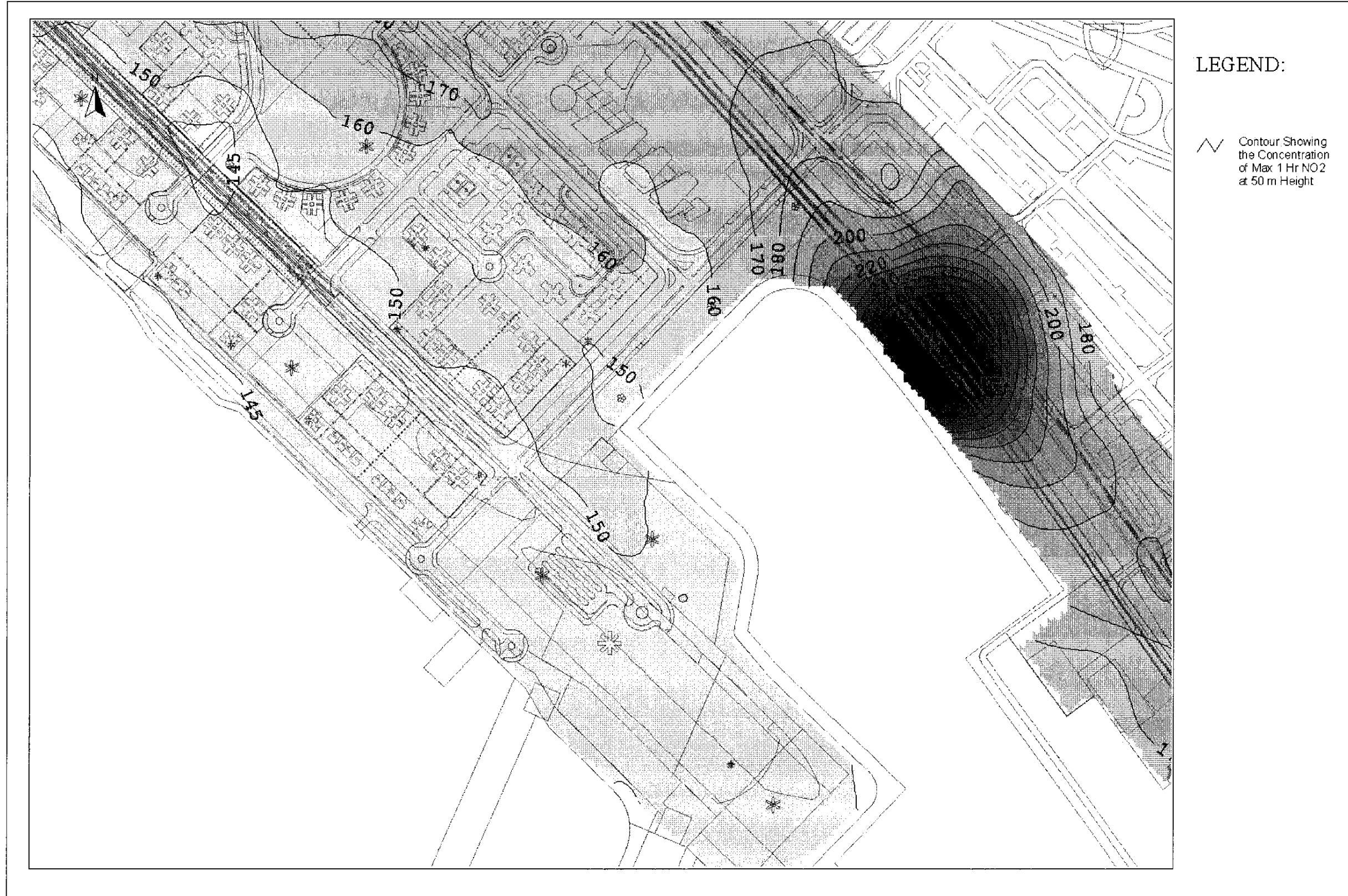
Drawing No. 22936/EN/319F Predicted Worst-case 1-hr Average NO 2 Concentration Contours at 50m Above Ground
