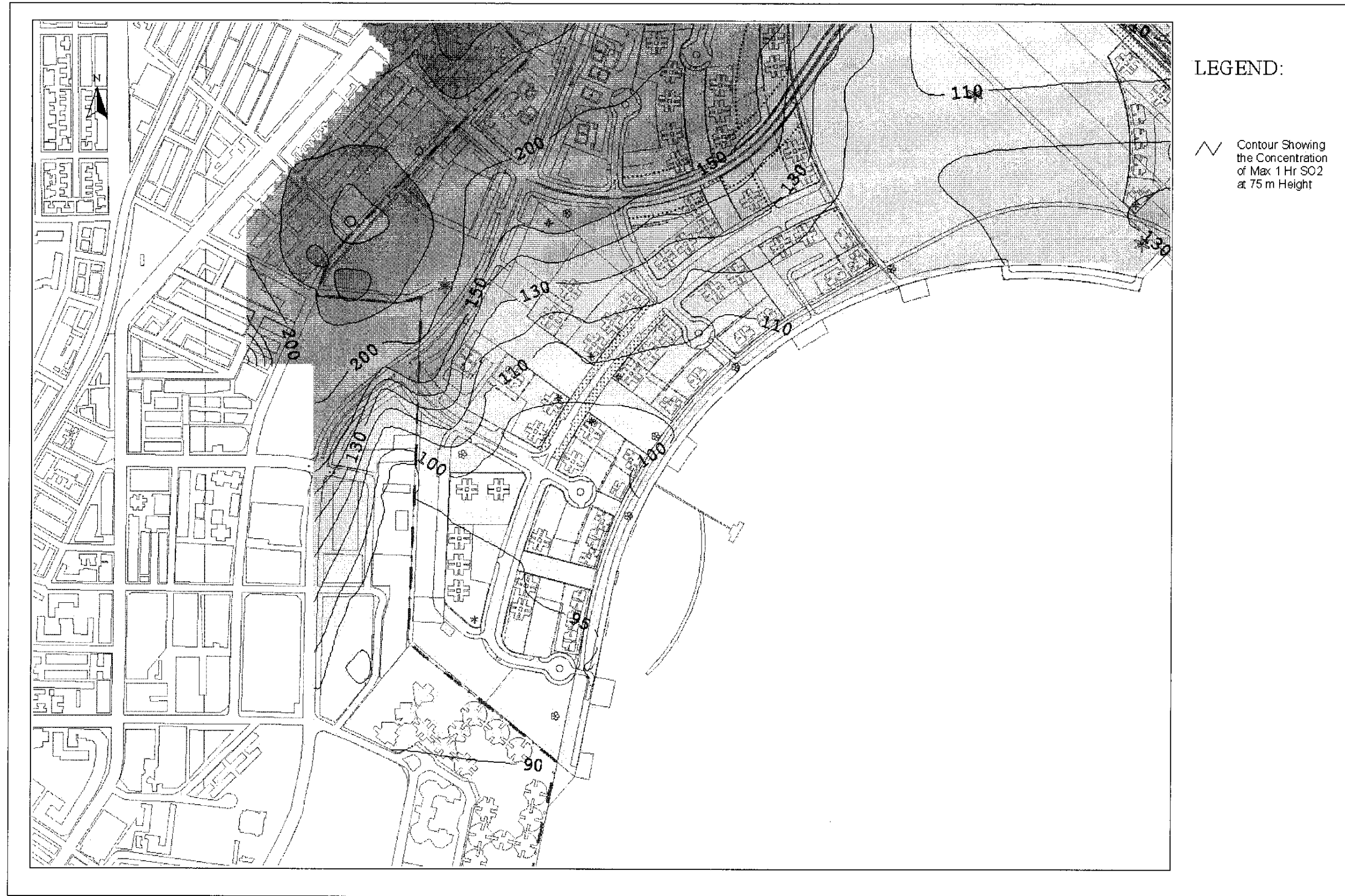
Drawing No. 22936/EN/331D Predicted Worst-case 1-hr Average SO 2 Concentration Contours at 75m Above Ground
