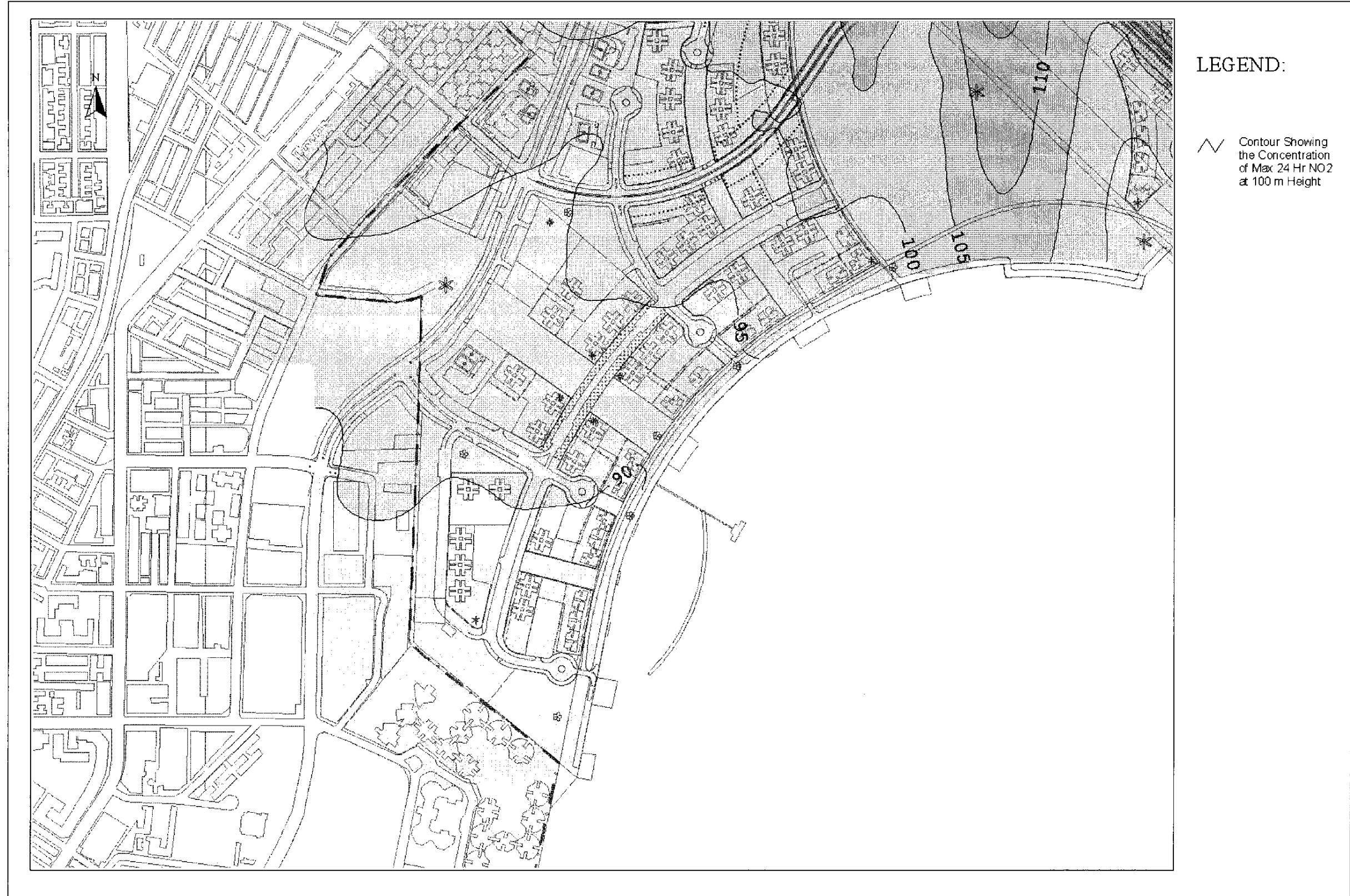
Drawing No. 22936/EN/327D Predicted Worst-case 24-hr Average NO 2 Concentration Contours at 100m Above Ground
