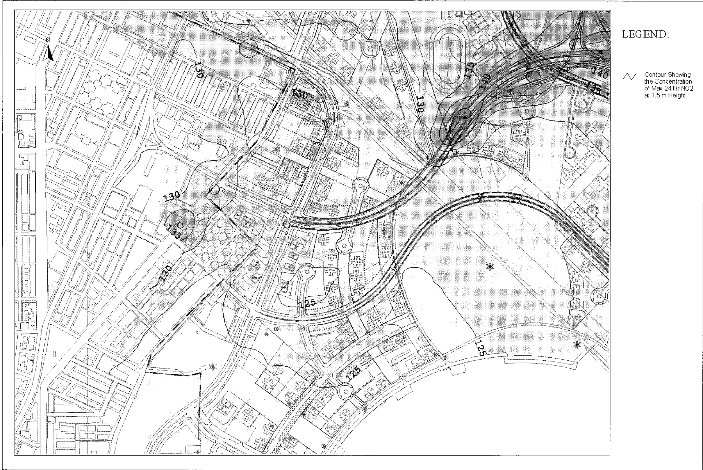
Drawing No. 22936/EN/322C Predicted Worst-case 24-hr Average NO 2 Concentration Contours at 1.5m Above Ground
