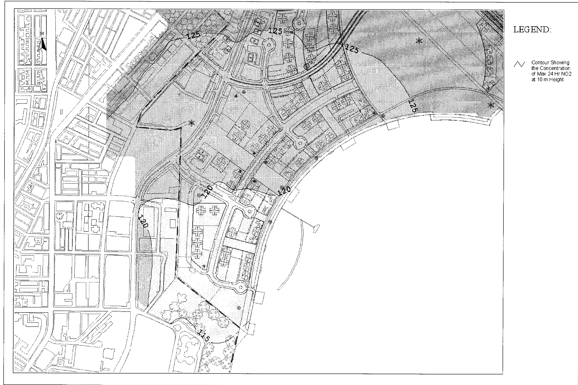
Drawing No. 22936/EN/323D Predicted Worst-case 24-hr Average NO 2 Concentration Contours at 10m Above Ground
