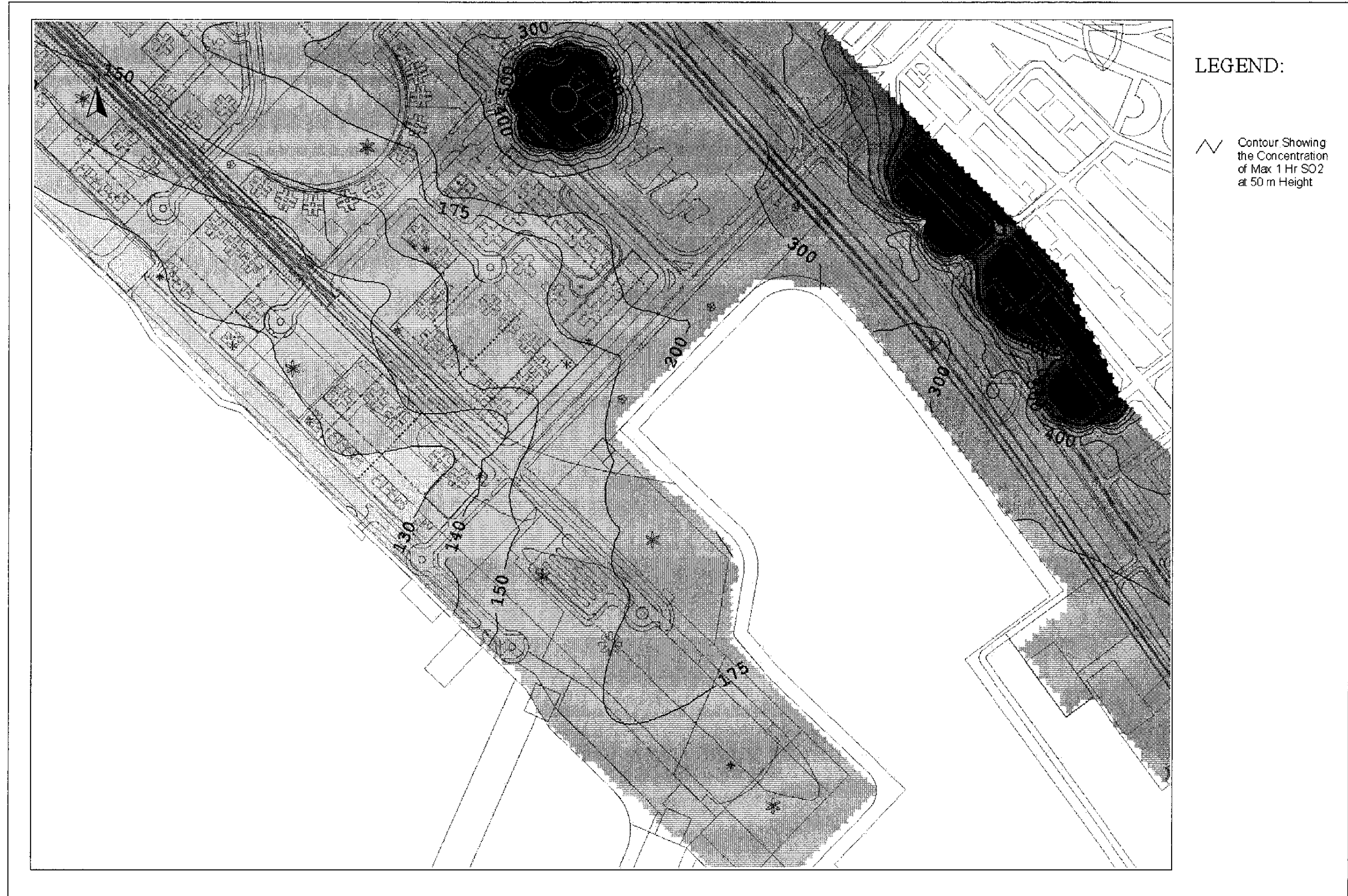
Drawing No. 22936/EN/330F Predicted Worst-case 1-hr Average SO 2 Concentration Contours at 50m Above Ground
