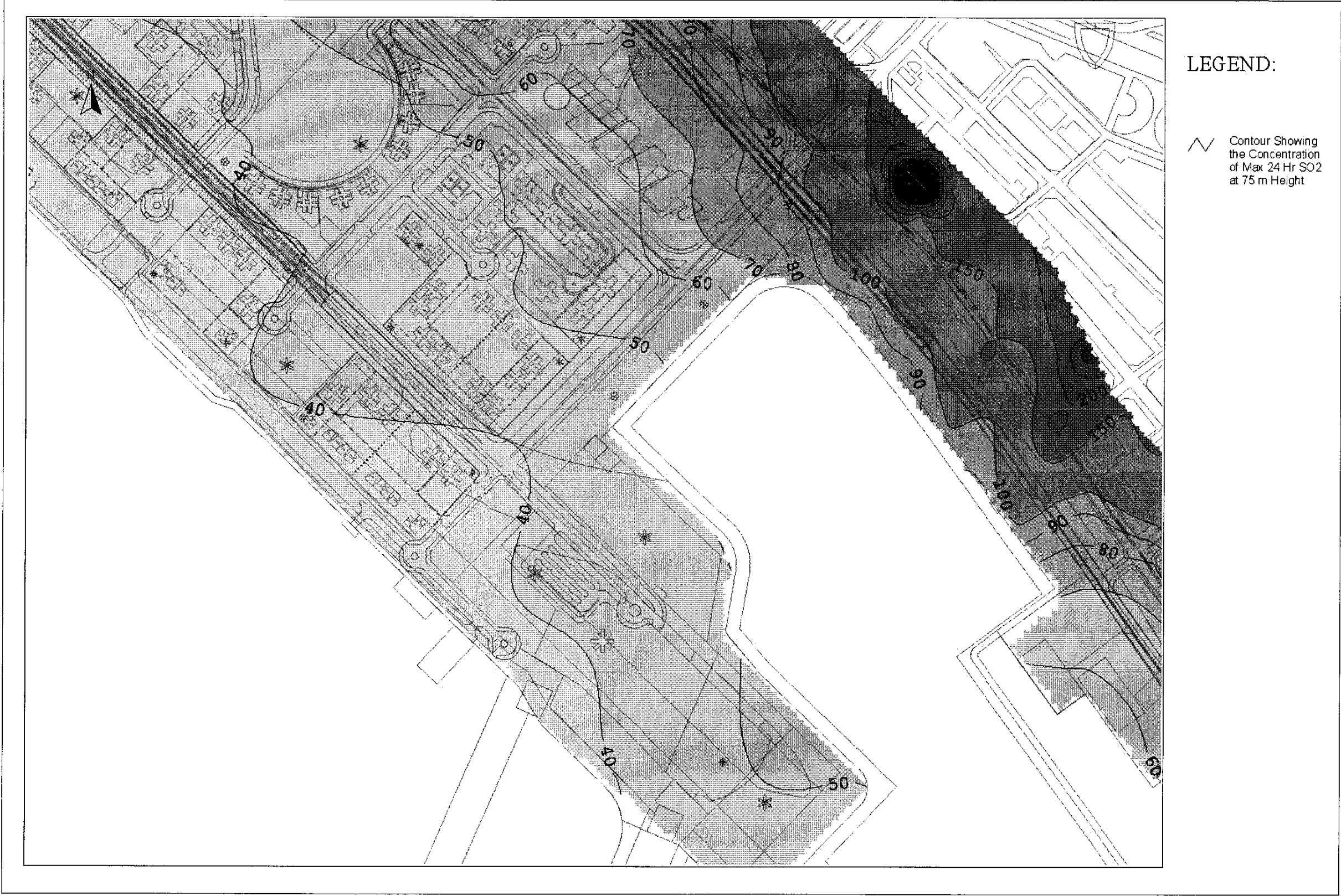
Drawing No. 22936/EN/335F Predicted Worst-case 24-hr Average SO 2 Concentration Contours at 75m Above Ground
