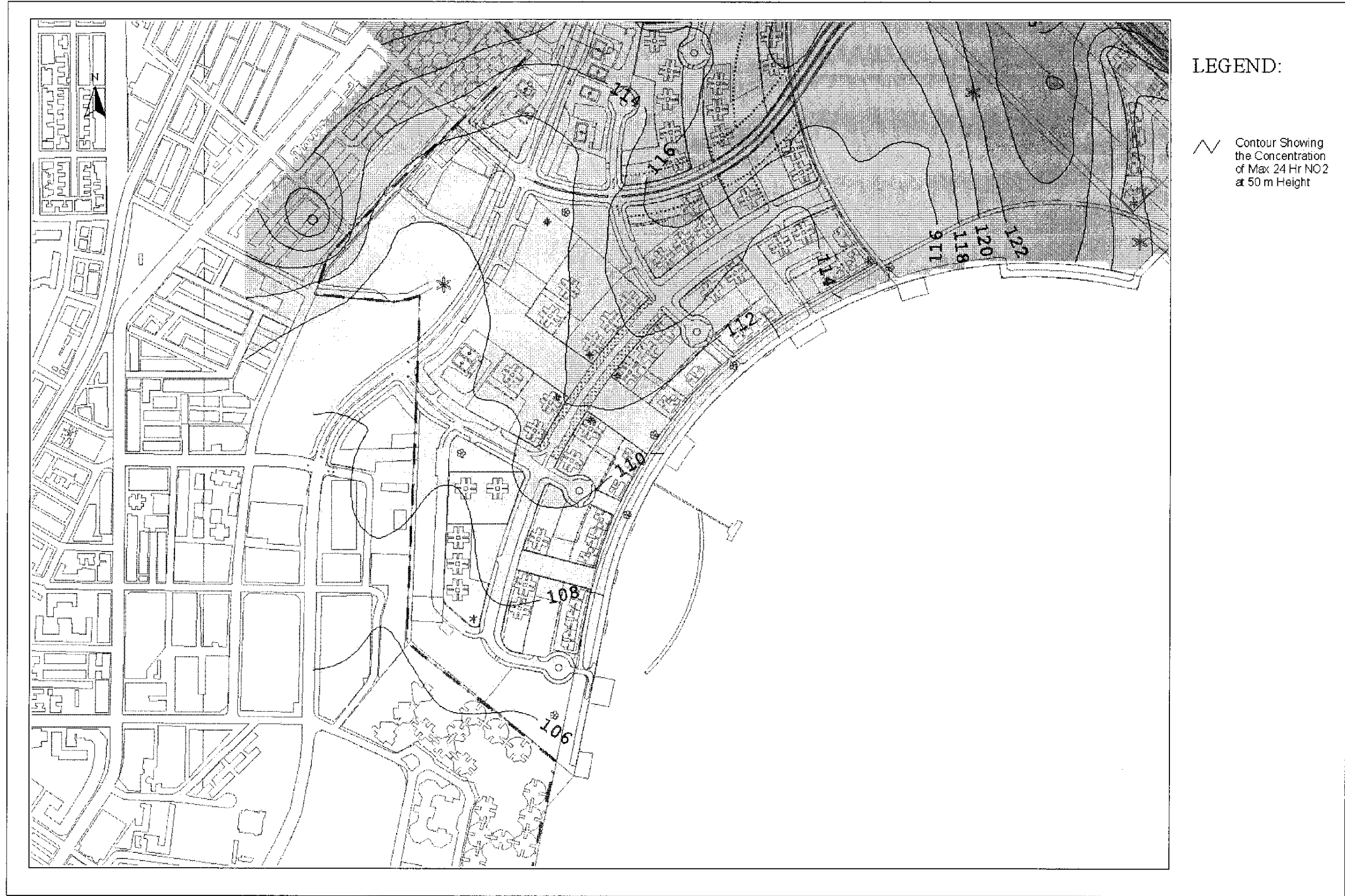
Drawing No. 22936/EN/325D Predicted Worst-case 24-hr Average NO 2 Concentration Contours at 50m Above Ground
