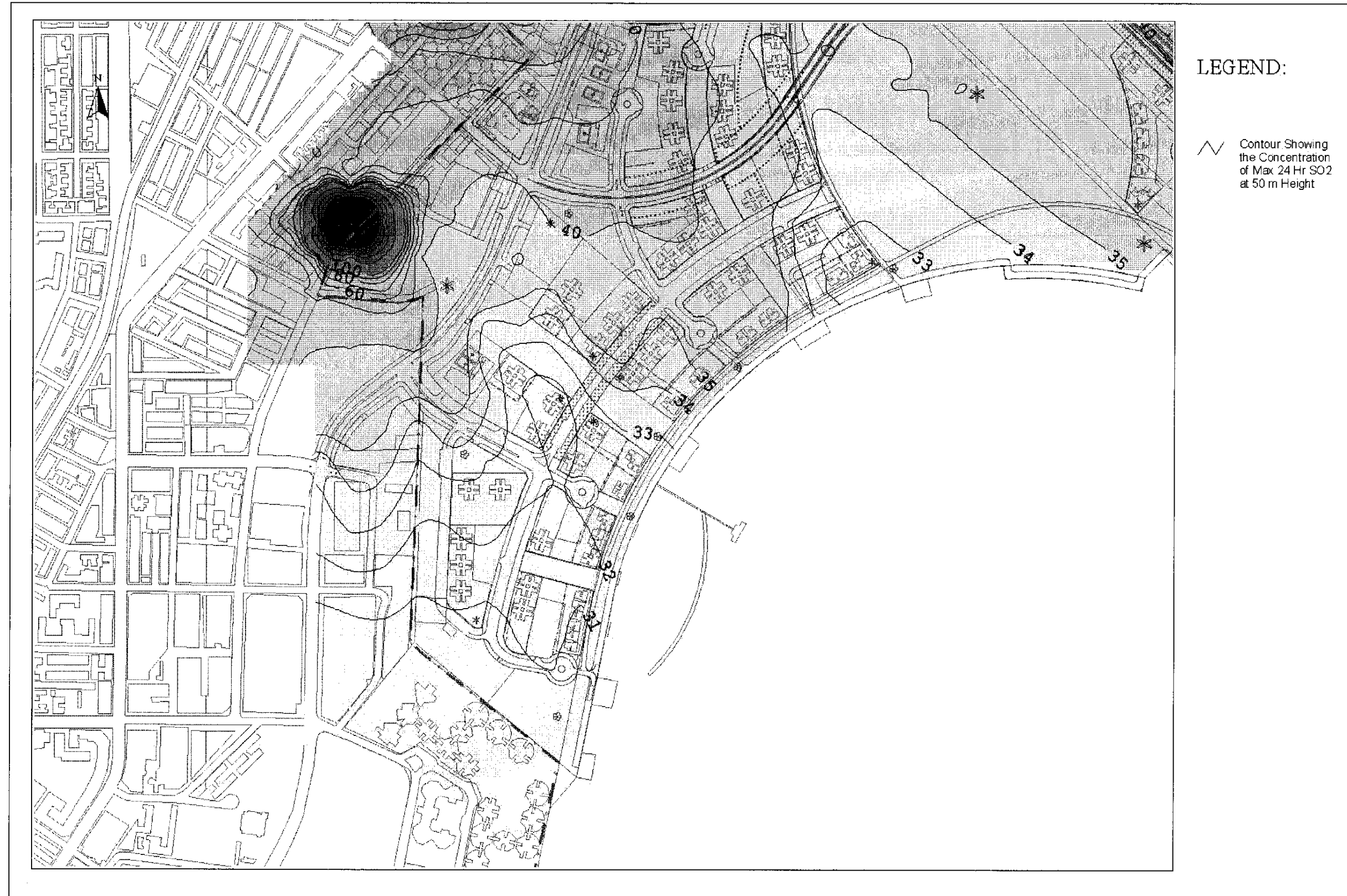
Drawing No. 22936/EN/334D Predicted Worst-case 24-hr Average SO 2 Concentration Contours at 50m Above Ground
