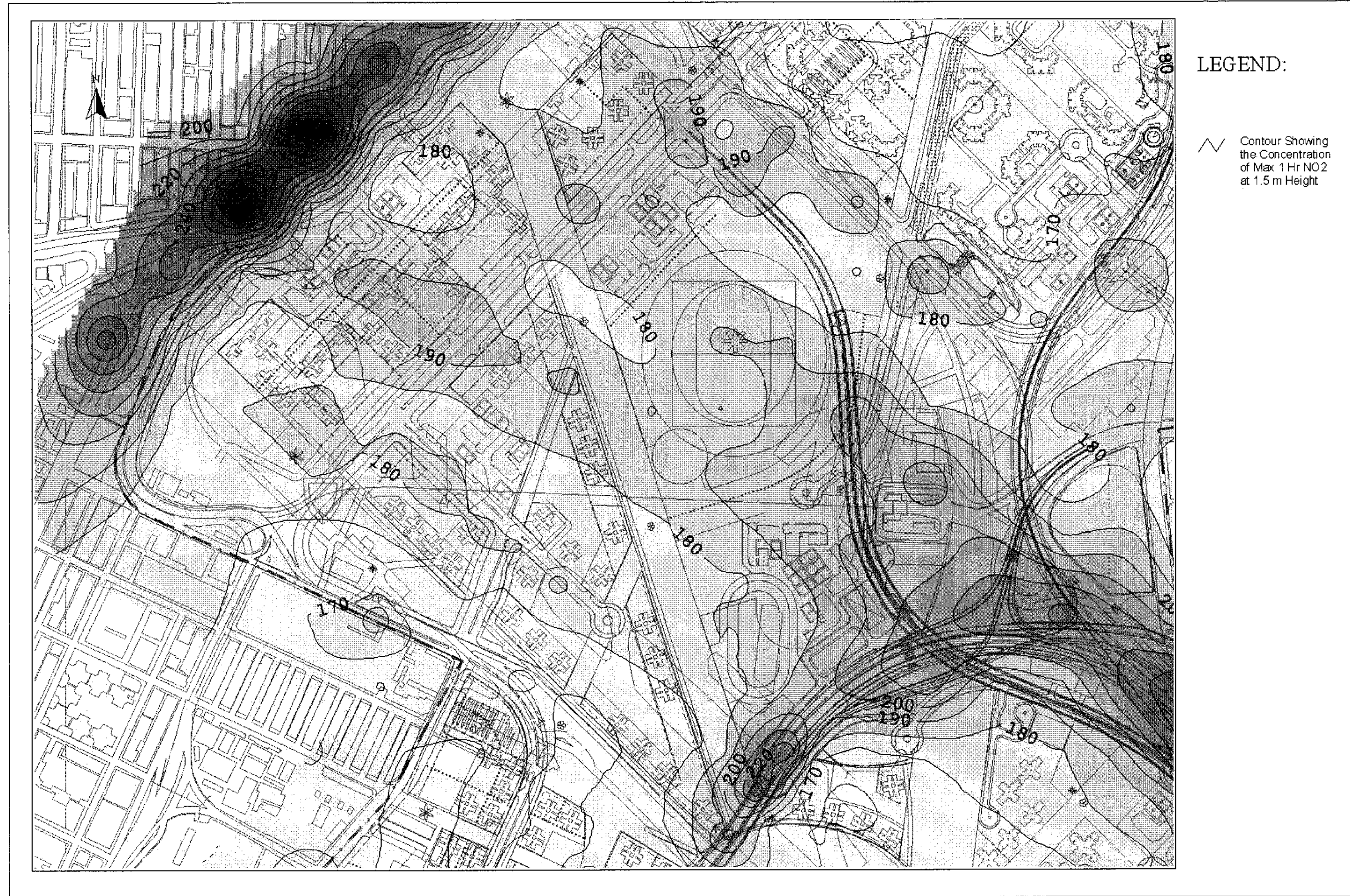
Drawing No. 22936/EN/316B Predicted Worst-case 1-hr Average NO 2 Concentration Contours at 1.5m Above Ground
