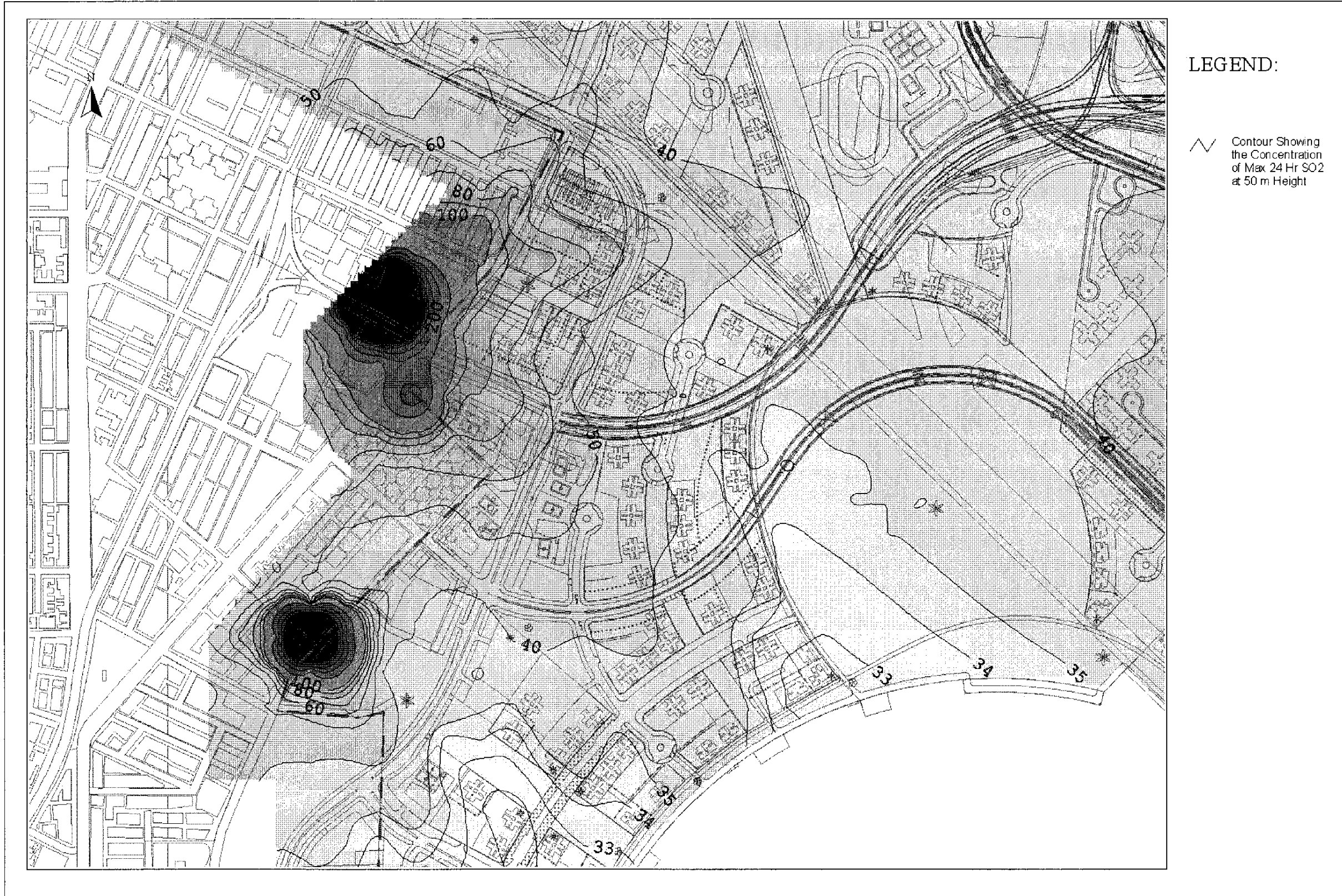
Drawing No. 22936/EN/334C Predicted Worst-case 24-hr Average SO 2 Concentration Contours at 50m Above Ground
