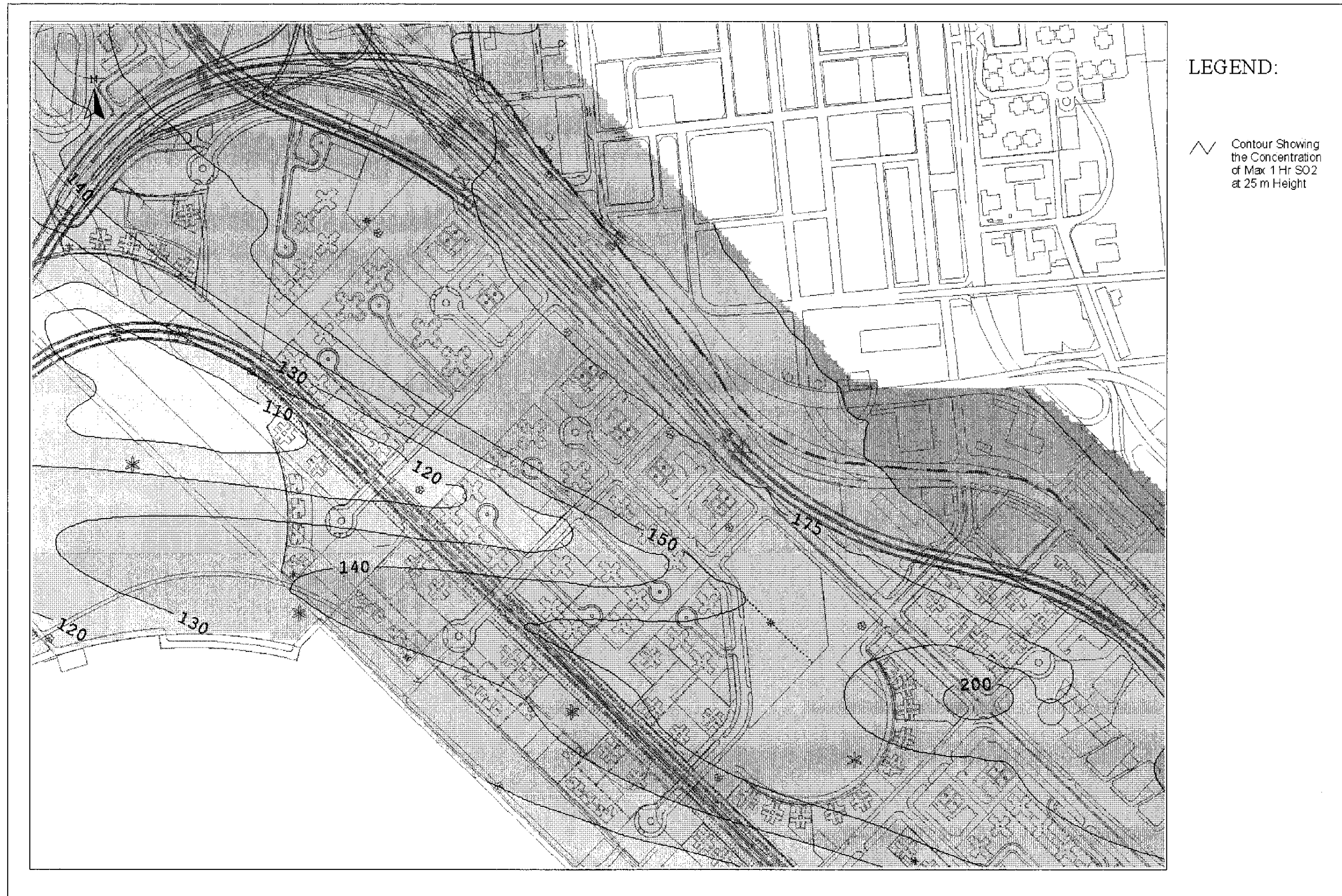
Drawing No. 22936/EN/329E Predicted Worst-case 1-hr Average SO 2 Concentration Contours at 25m Above Ground
