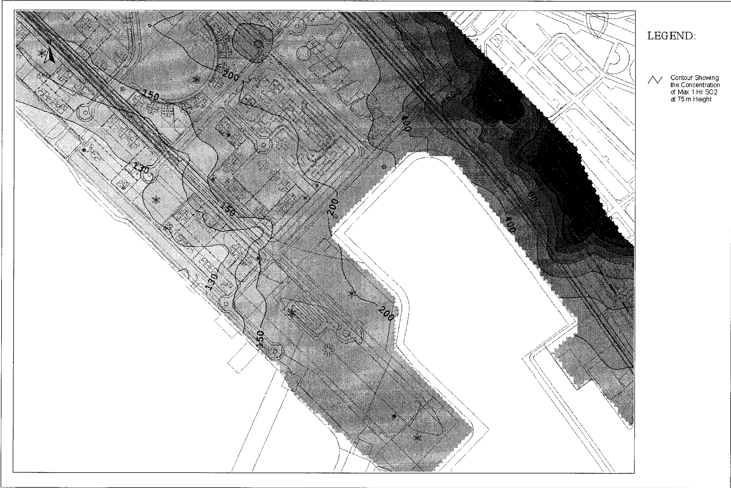
Drawing No. 22936/EN/331F Predicted Worst-case 1-hr Average SO2 Concentration Contours at 75m Above Ground
