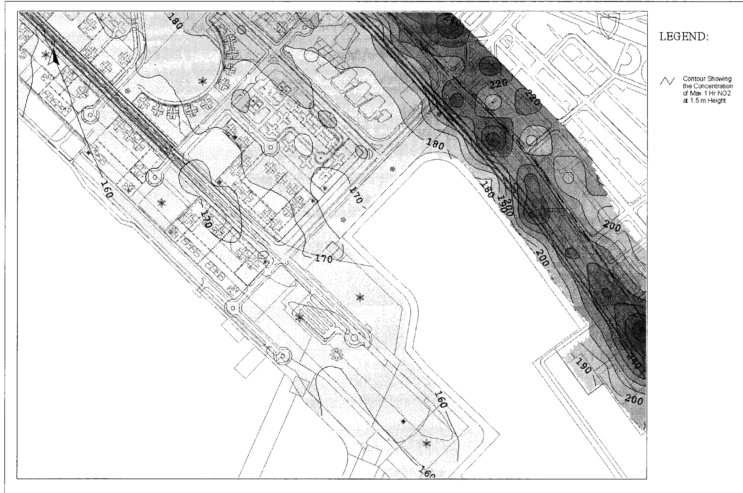
Drawing No. 22936/EN/316F Predicted Worst-case 1-hr Average NO 2 Concentration Contours at 1.5m Above Ground
