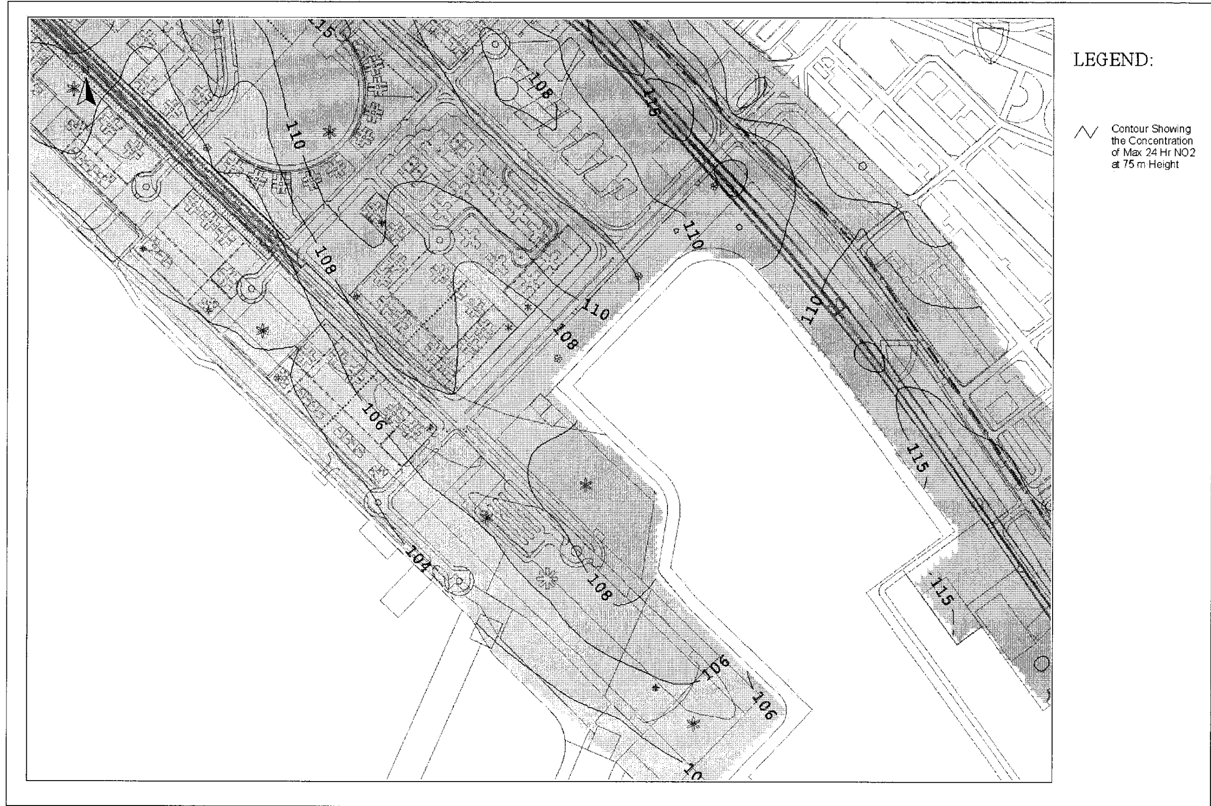
Drawing No. 22936/EN/326F Predicted Worst-case 24-hr Average NO 2 Concentration Contours at 75m Above Ground
