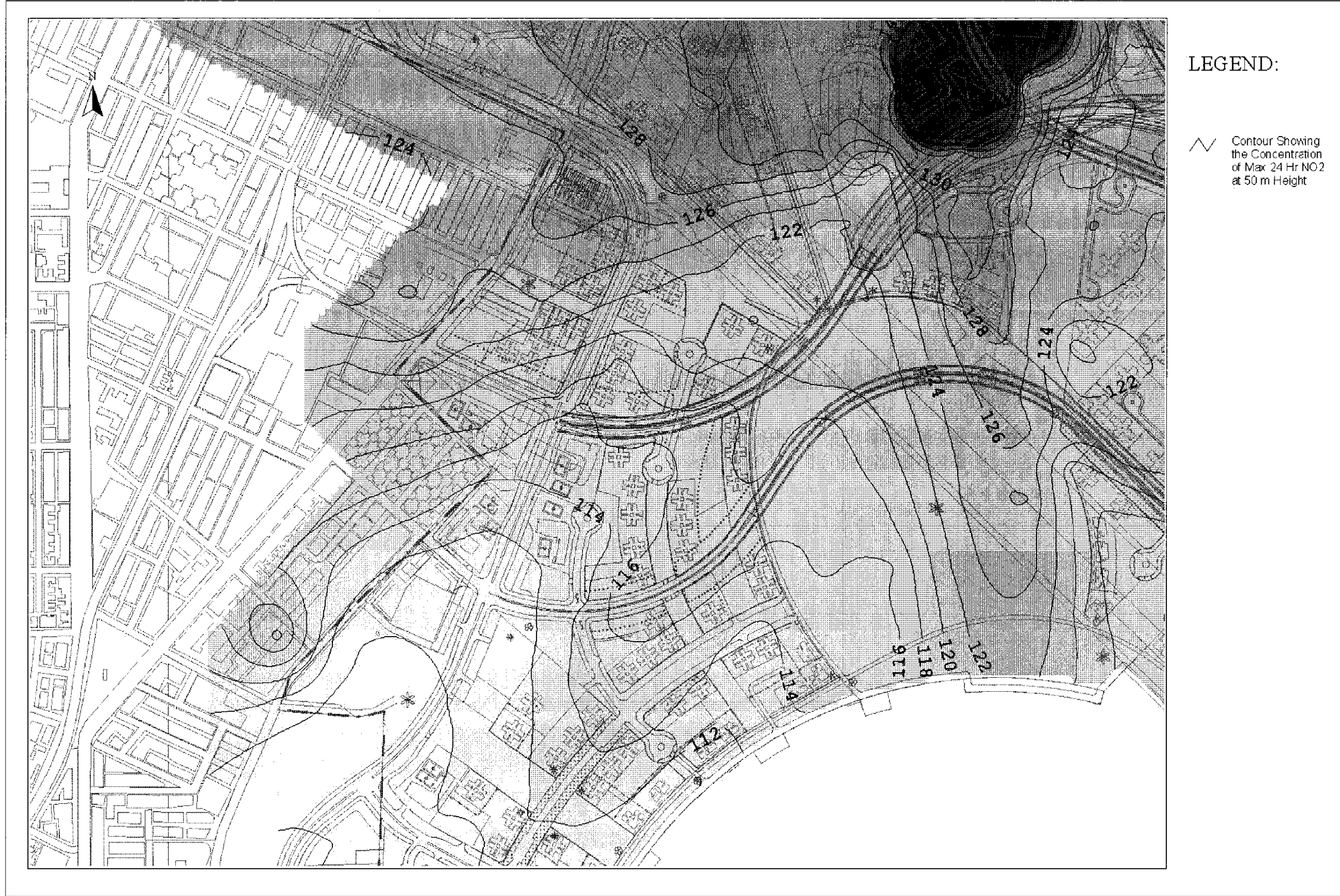
Drawing No. 22936/EN/325C Predicted Worst-case 24-hr Average NO 2 Concentration Contours at 50m Above Ground
