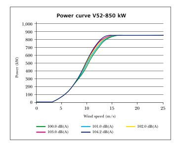
The figure above illustrates the power curves at different sound levels for the V52-850 kW turbine, which is equipped with OptiSpeed<sup>®</sup>.
